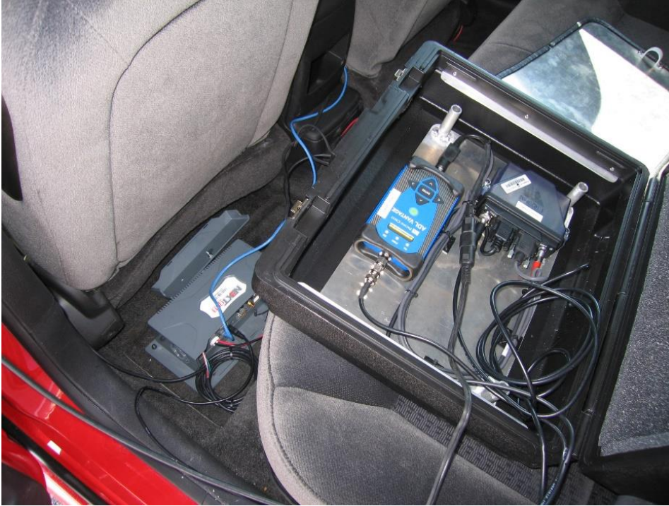
Figure 3-2. Data acquisition testing kit installed in the vehicle's back seat.
