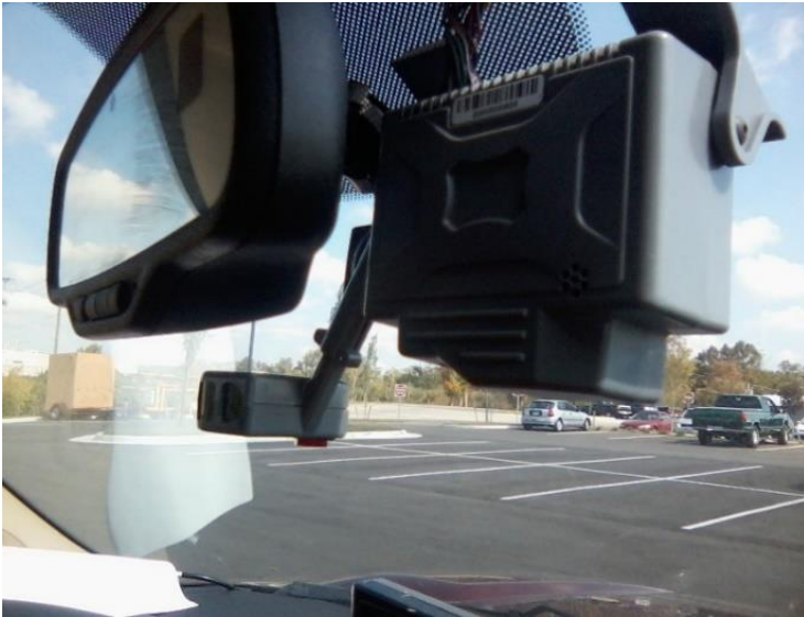
Figure 3-4. Head unit installed on windshield.
