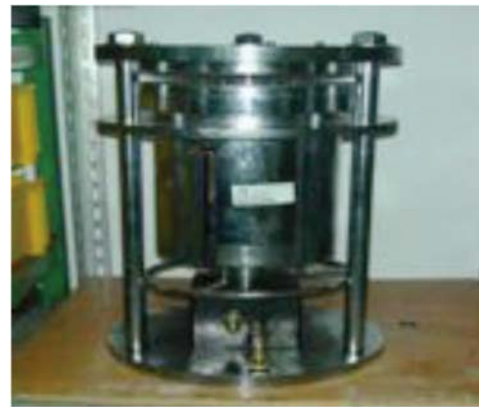
(b) ASTM D6241 (CBR) hydraulic puncture apparatus (Hsieh and Wang (2008))
