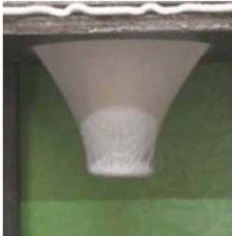
Figure 2.10. Failure stages of polyester needlepunched nonwoven geotextile (Askari, Najjar et al. 2012).
