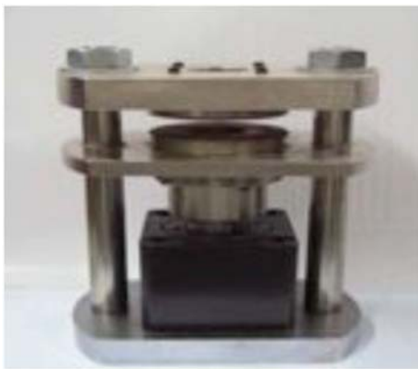
(a) ASTM D4833 (pin) hydraulic puncture apparatus (Hsieh and Wang (2008))
