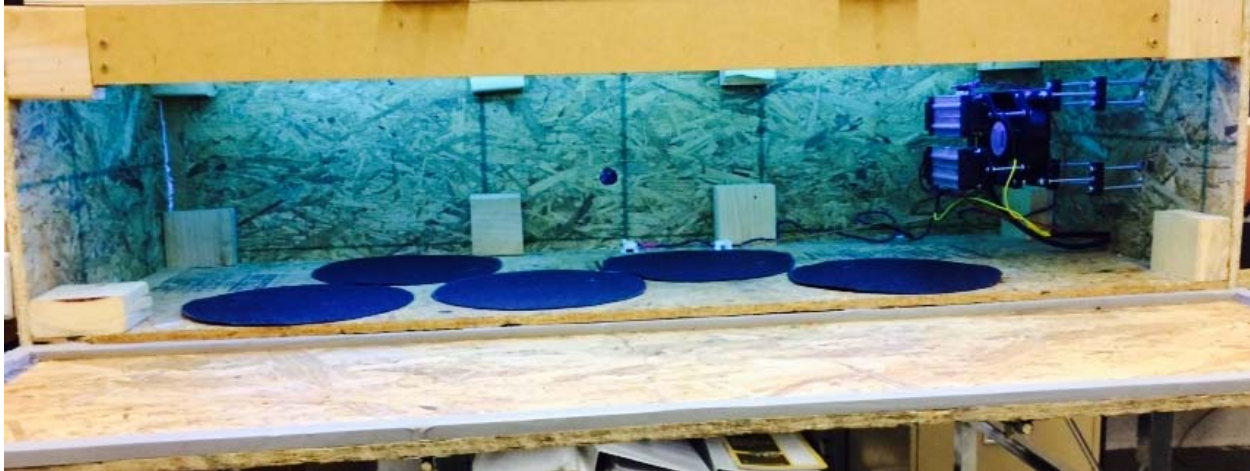
Figure 3.10 Geotextile specimens in UV chamber at UW-Milwaukee with UV340B lamps and pair of 500W ceramic heaters.
