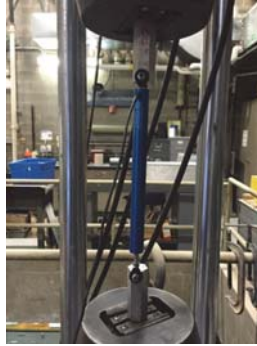
Fig. 57. The installation of the sensor head on the loading frame.
