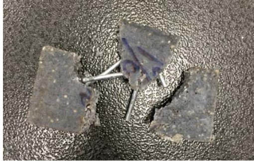
Fig. 68. Elastomeric concrete specimen (1% reinforcement) after impact
