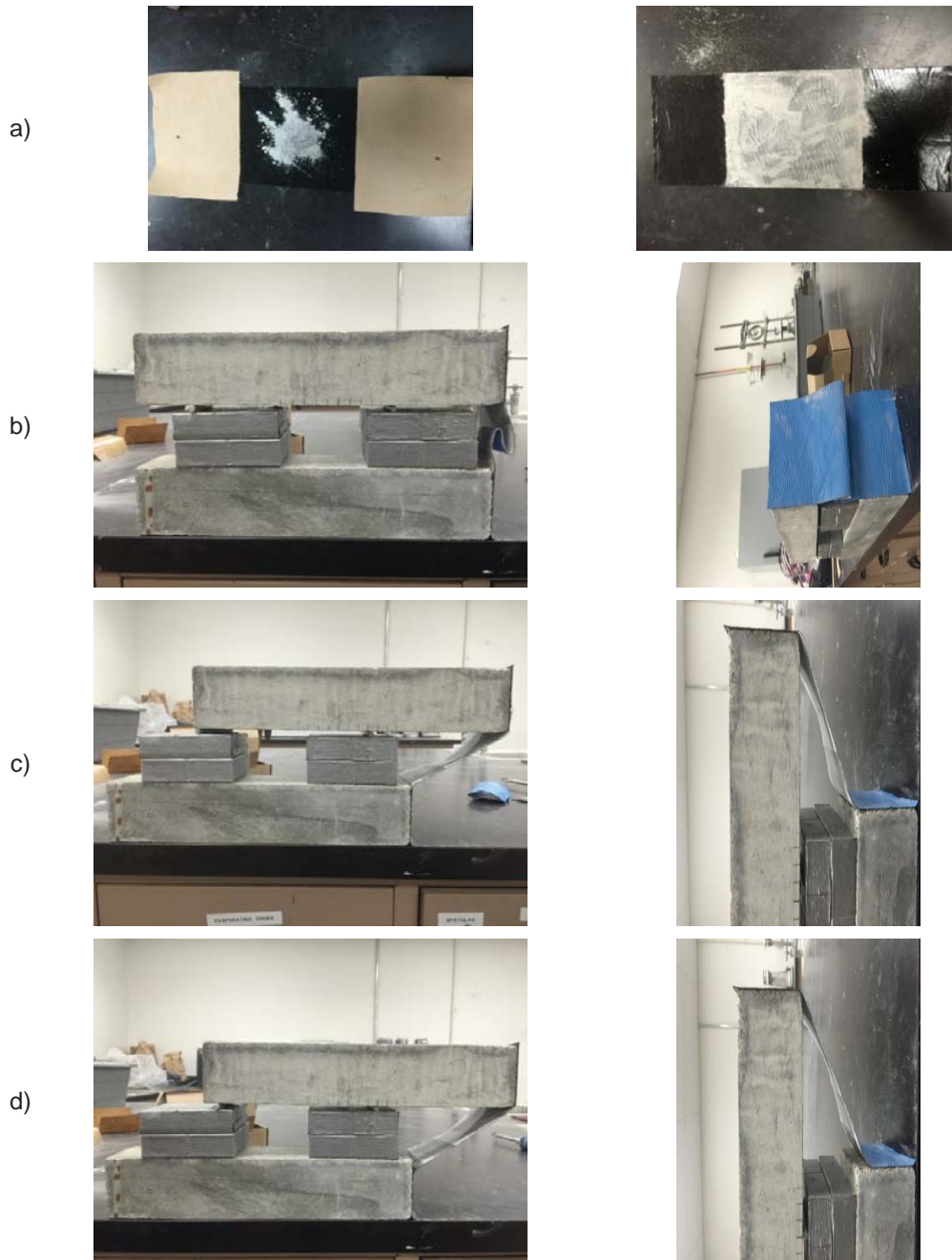
Fig. 49. Experiment of waterproof membrane with an overlap treated with shredded fiberglass powder: a) treatment of shredded fiberglass powder; b) overlap formed at the gap; c) no delamination at 2.8 in. slip; and d) delamination appears at 3.2 in. slip.
