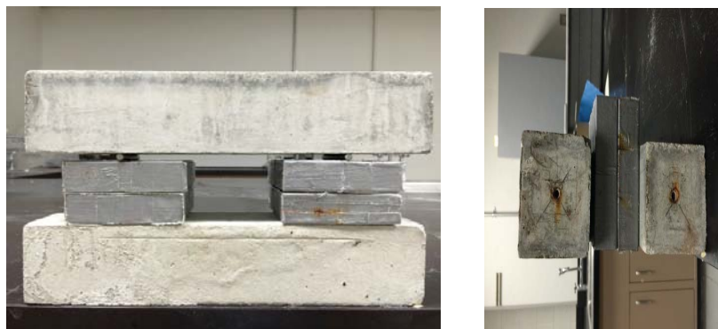
Fig. 46. Experimental setup for the out-of-plane shear test.
