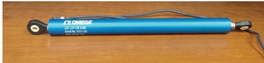
Fig. 53. LDI-119-150-A20A sensor head procured from OMEGA Engineering.
