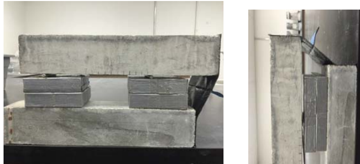
Fig. 48. Delamination of waterproof membrane with a double layer formed by self-stickness.
