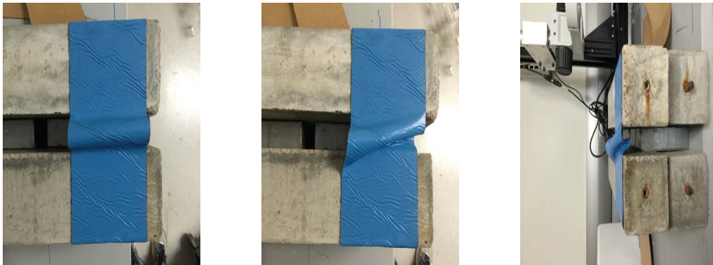
Fig. 52: In-plane shear of the waterproof membrane with a treated overlap.
