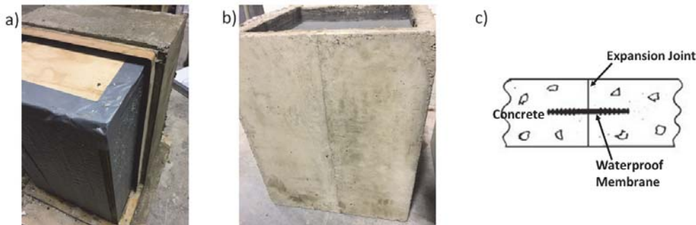
Fig. 41. a) The implementation of a polymer-based waterstop in the water tank; b) the water tank during test; and c) Illustration of the implementation of the polymer-based waterstop.
