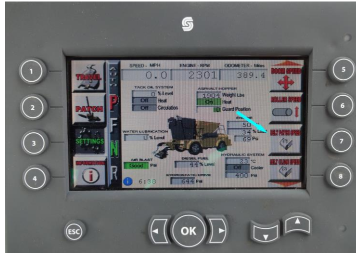
Figure 26. Asphalt Delivery Rate Setting
