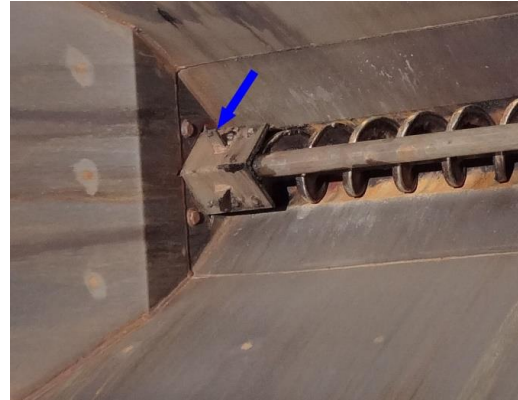
Figure 18. Python PHP Guard Fins
