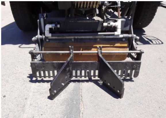
Figure 22. Python PHP Rake & Funnel Attachment
