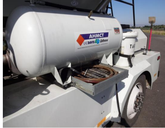
Figure 12. Python PHP Fill Hose Tray and Bucket
