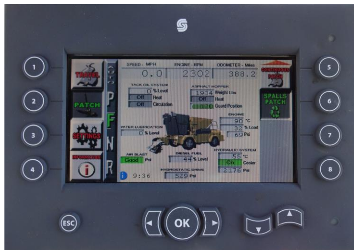
Figure 43. Spall Repair Screen
