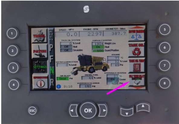
Figure 15. Settings Screen – Belt Delay
