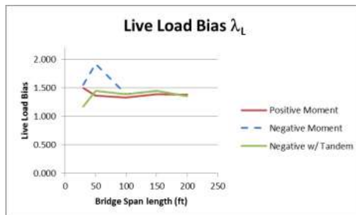
Figure 14. Live Load Bias with Commentary Low-boy Tandem Loading
