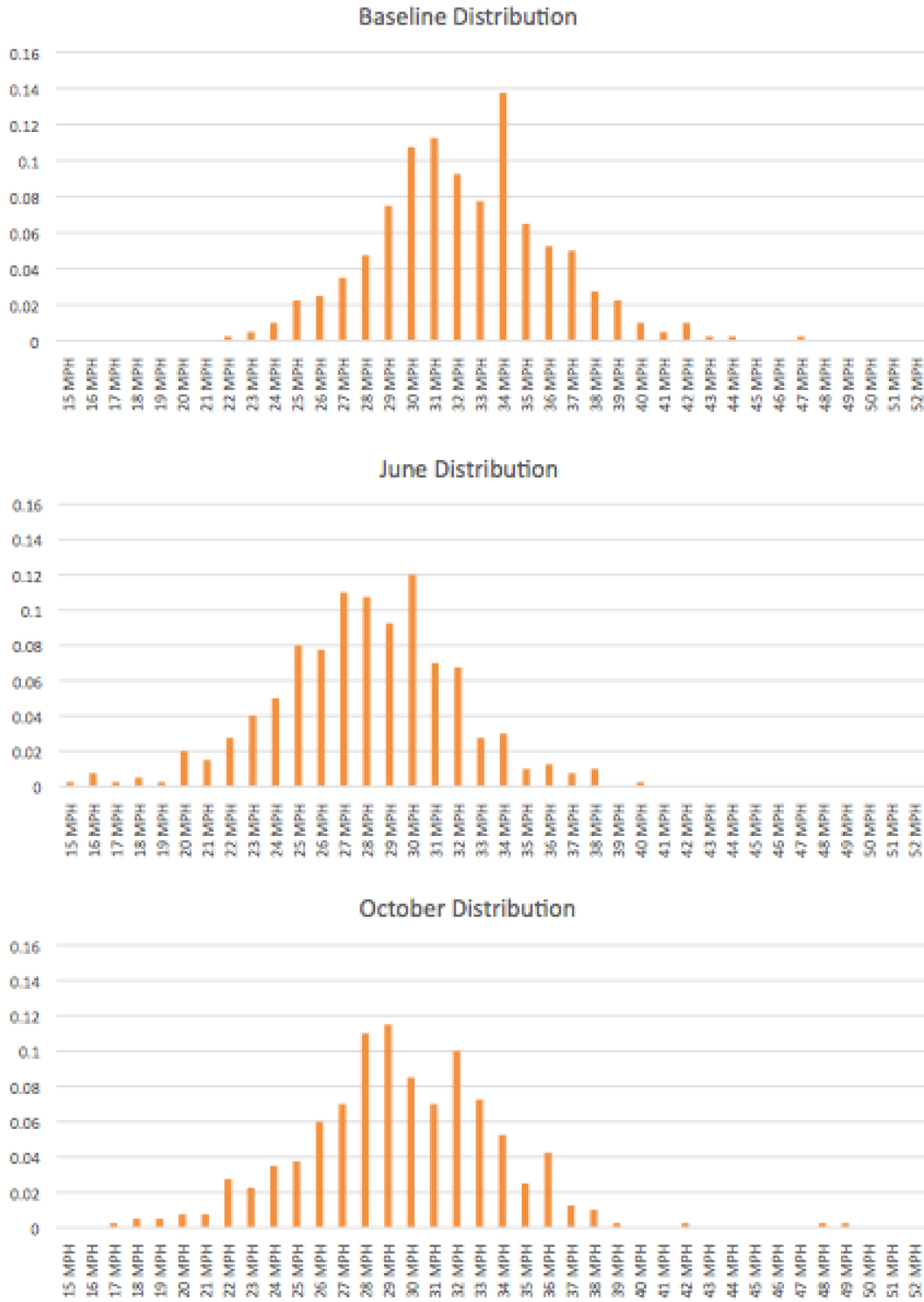
Figure 4.1 Speed distribution at the crosswalk for Nixon at Bluett. The top frame shows the distribution of speeds for baseline, the middle frame shows the distribution in June and the bottom frame shows the distribution in October.
