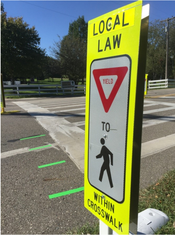
Figure 5.2 Photograph of crosswalks with tape lines marking placement of sign for each gateway width.
