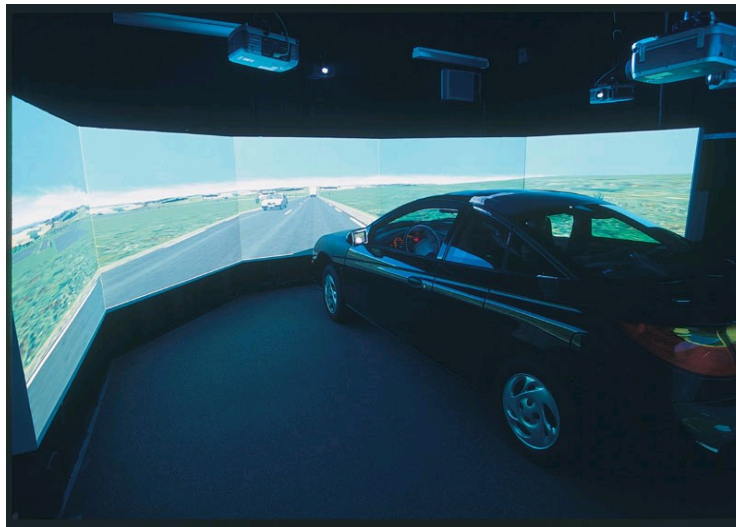
Figure 4.1 HumanFIRST immersive driving simulator.
