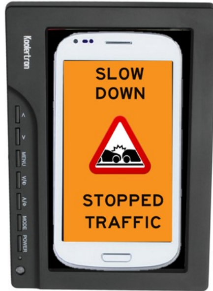
Figure 4.2 LCD screen used to deliver work zone messages.
