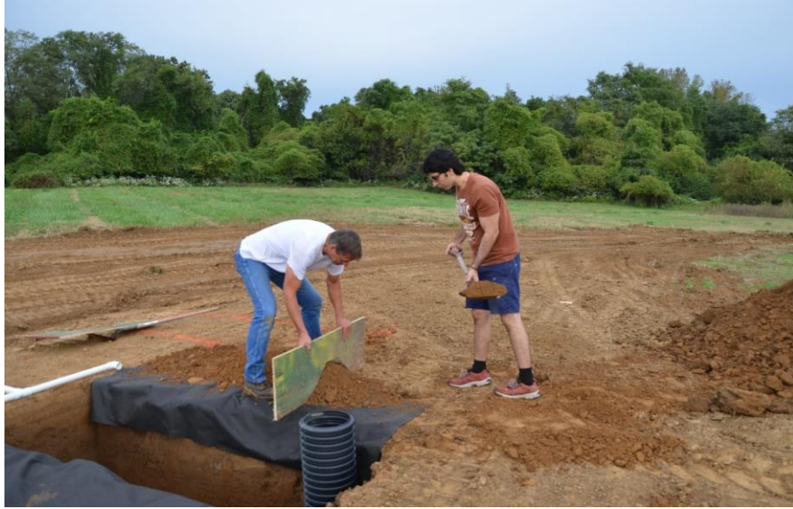
Figure 41. A test cell with observation well and protection fiber.
