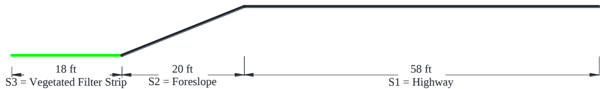
Figure 32. Vegetated filter strip draining an idealized catchment.
