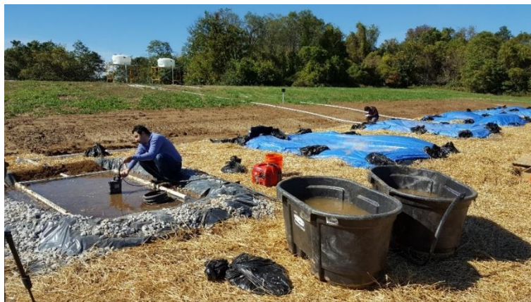
Figure 51. Pumping run-off into the collecting tanks.
