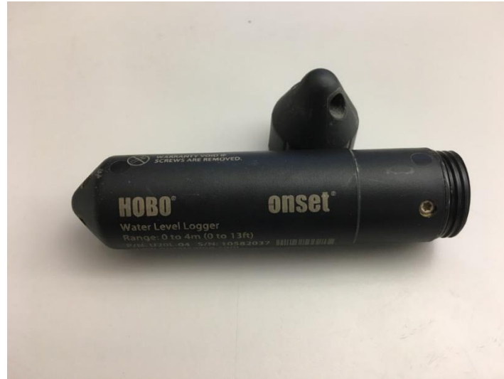
Figure 50. Pressure sensor used to measure water depth.
