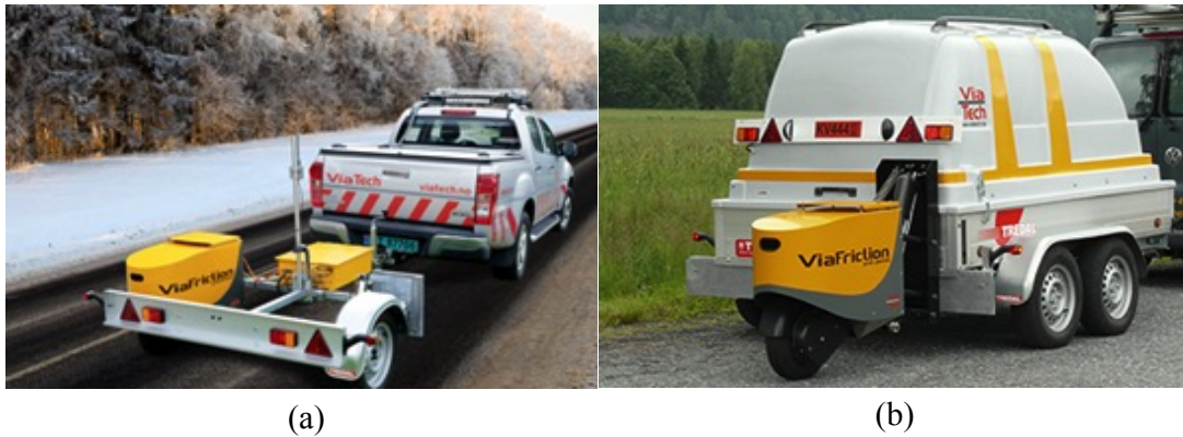
Figure 21. ViaFriction Winter Trailer: (a) Without Water System and (b) With Water System
