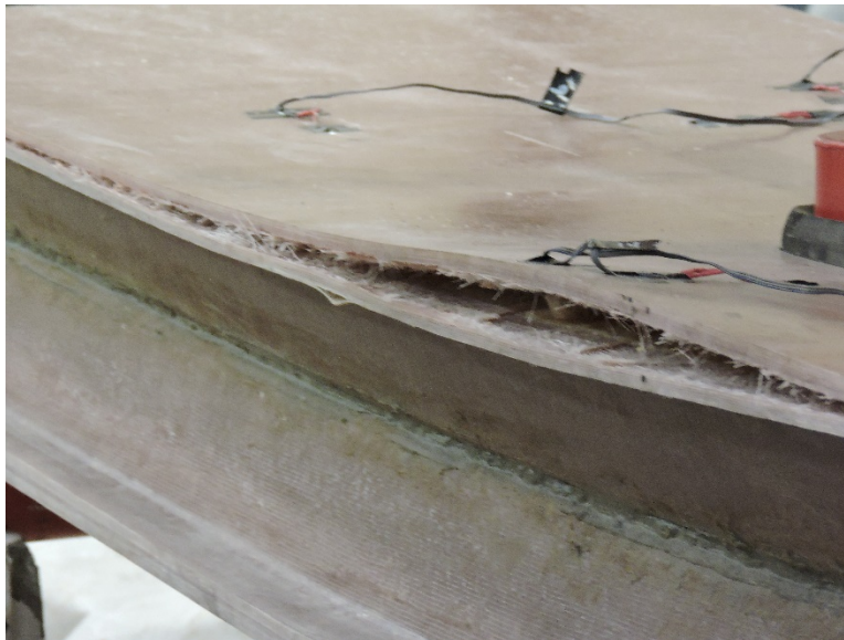
Figure 3.12: Local Buckling of Compression Flange, Specimen FP-1
