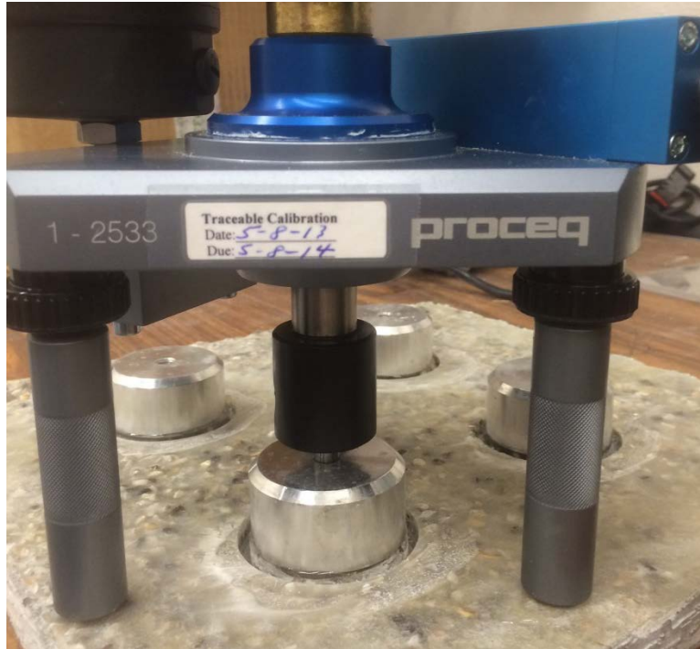
Figure 7.11: Direct Pull-off Bond Testing of Overlay Materials
