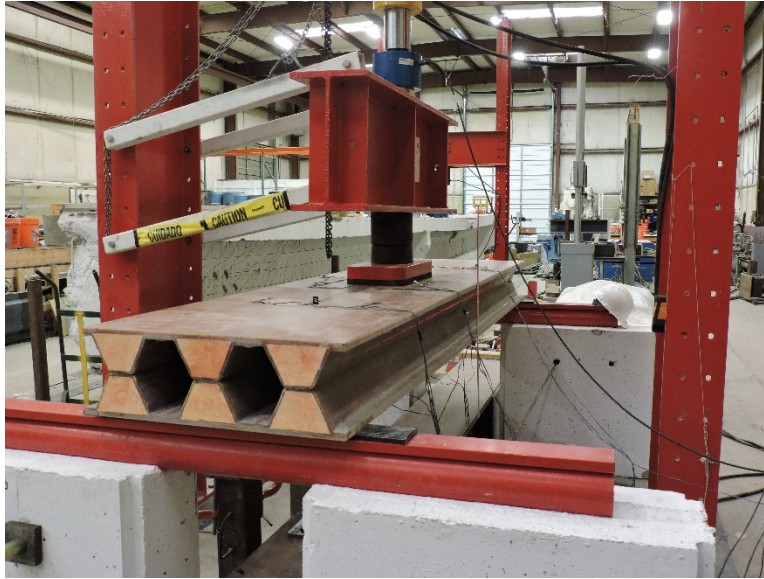
Figure 3.4: Flexural Test Setup for FRP Deck Specimens
