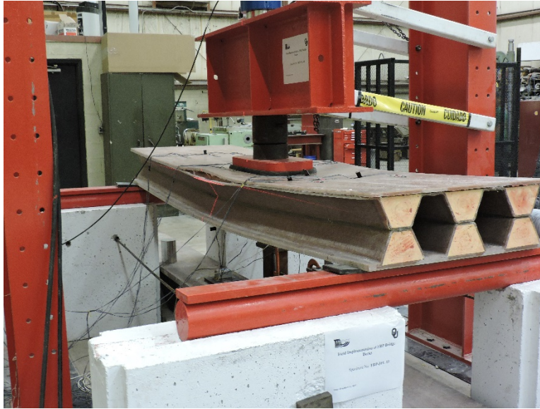
Figure 3.11: Local Buckling of Compression Flange, Specimen FP-1
