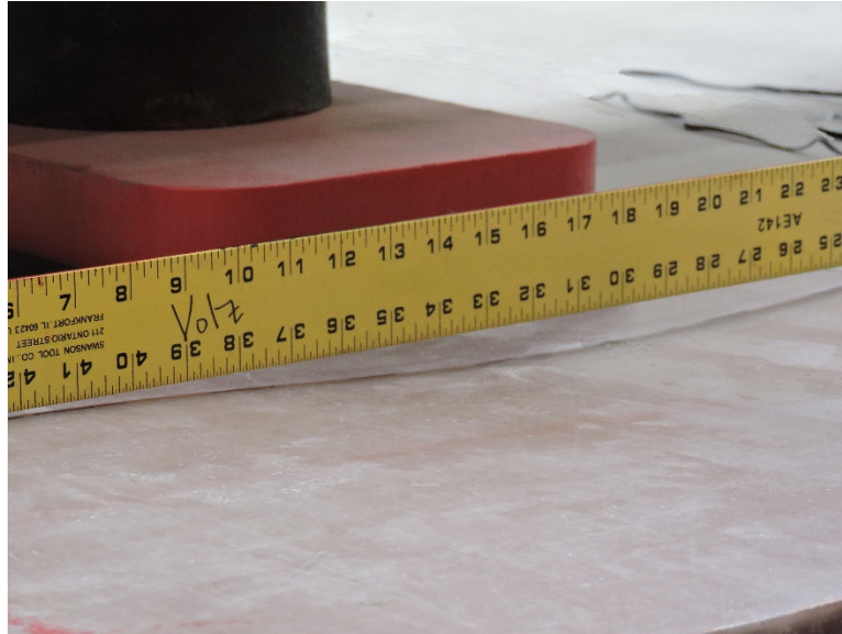
Figure 3.17: Top Facesheet Depressing Due to Buckled Web Below
