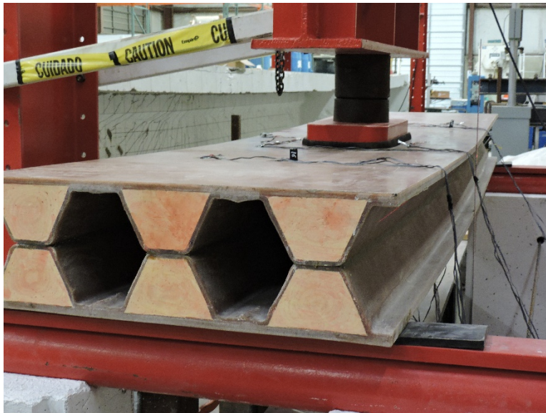
Figure 3.10: Specimen FP-1 During Flexural Test, 75 kip Load
