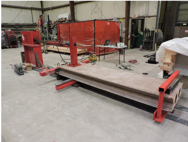
Figure 5.3: Guardrail-to-Panel Connection Test Setup for FRP Deck Specimens
