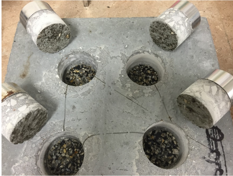
Figure 7.15: Bond Failure at Interface of T-18 and LMC
