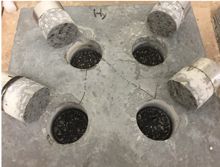
Figure 7.14: Bond Failure at Interface of T-48 and LMC
