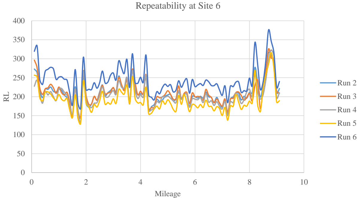
Figure 34: Vertical offsetting at site 6.
