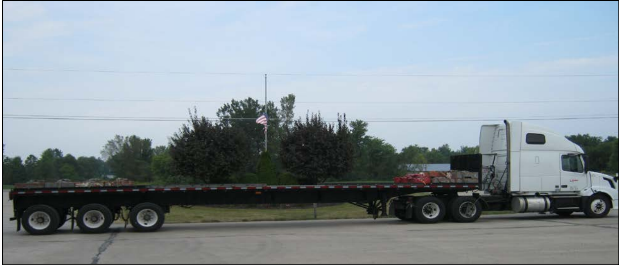
Figure 1. Photo. Test vehicle in 80,000-lb GVW configuration.
