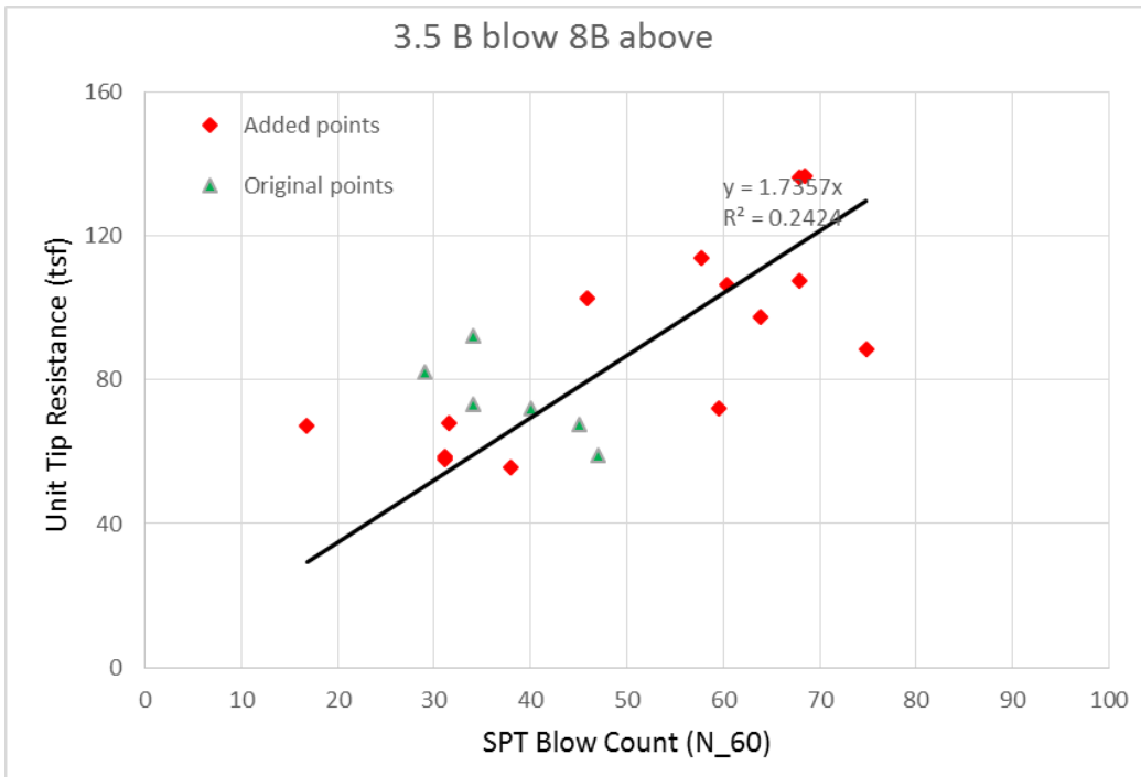
Figure 4.8 PCP in competent limestone – Averaging SPT N, 3.5B below and 8B above
