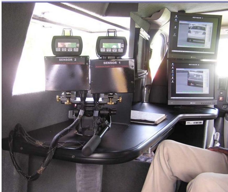
Figure 6.28 Mobile Van with Cameras and Sensors for Photo Enforcement, Chattanooga, TN
