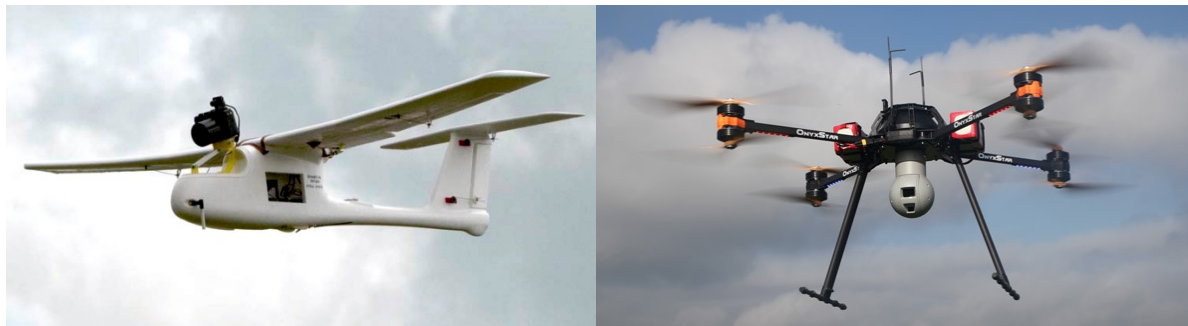
Figure 6.17 Fixed wing UAV (left) and Rotary wing UAV (right), both with cameras
