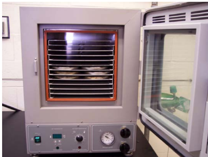
Figure 8. Vacuum Oven Aging to Simulate Long-Term Aging for Crack Sealants
