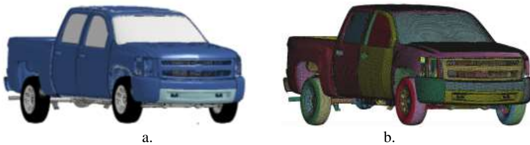
Figure 5. The FE models of a 2007 Chevy Silverado pickup (2270P). a. without mesh and b. with mesh [98].
