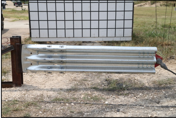
Figure 4.16. End Shoe before Test No. 490025-6 P6.
