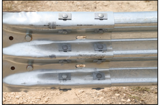
Figure 4.16. End Shoe before Test No. 490025-6 P6.
