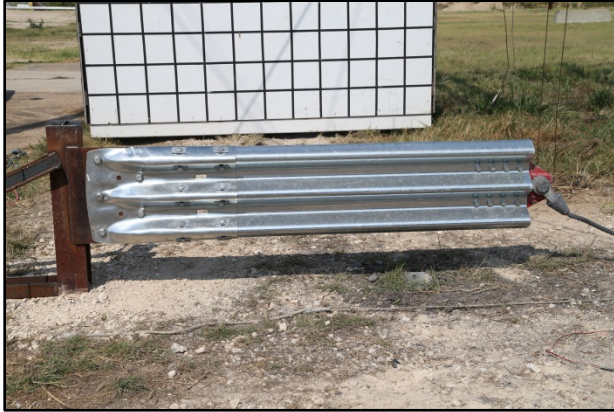
Figure 4.10. End Shoe before Test No. 490025-6 P4.
