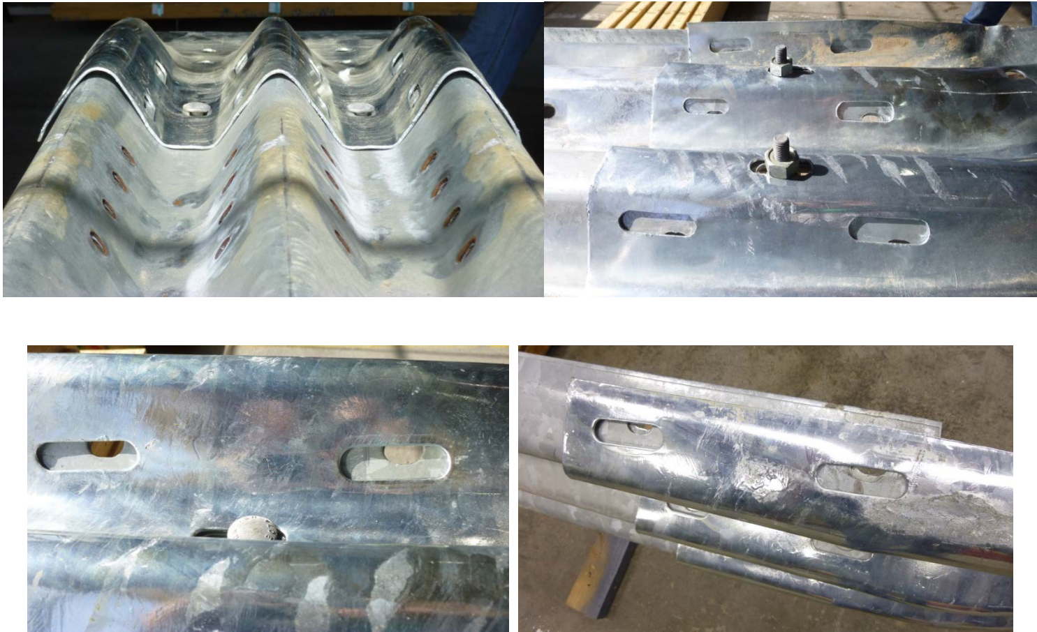
Figure 1.2. Misalignment of Slots Due to Geometrical Shifting.
