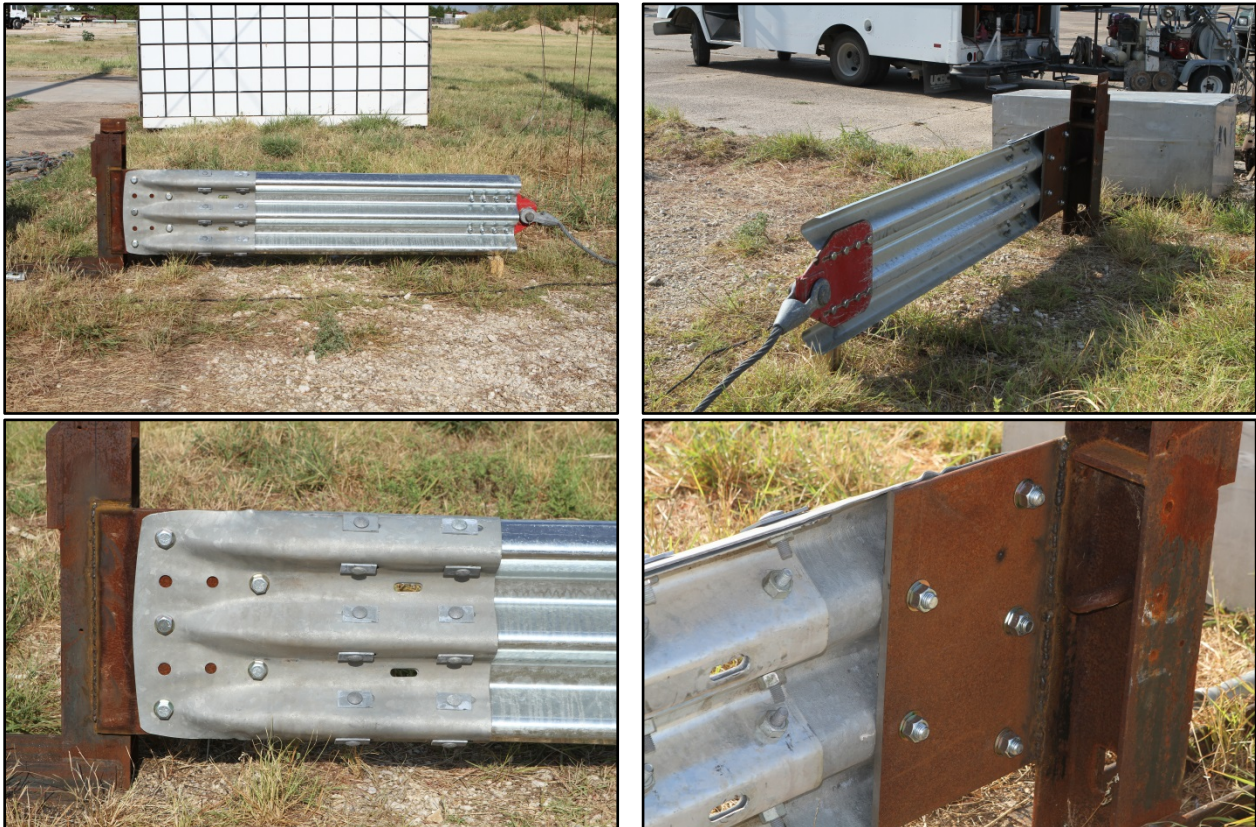
Figure 4.1. End Shoe before Test No. 490025-6 P1.
