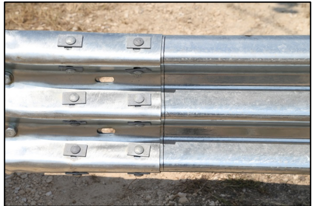
Figure 4.11. End Shoe after Test No. 490025-6 P4.
