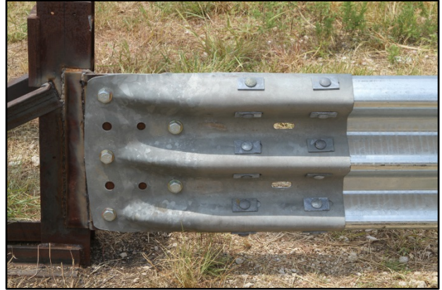
Figure 4.4. End Shoe before Test No. 490025-6 P2.
