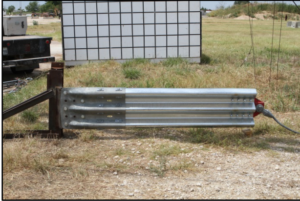
Figure 4.4. End Shoe before Test No. 490025-6 P2.
