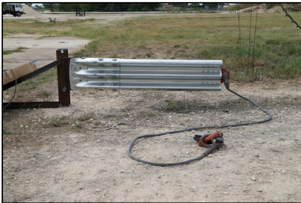
Figure 4.17. End Shoe after Test No. 490025-6 P6.
