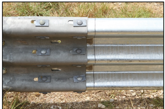
Figure 4.5. End Shoe after Test No. 490025-6 P2.
