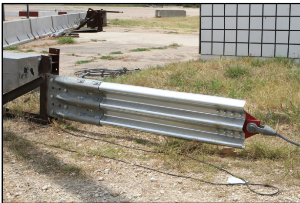
Figure 4.5. End Shoe after Test No. 490025-6 P2.
