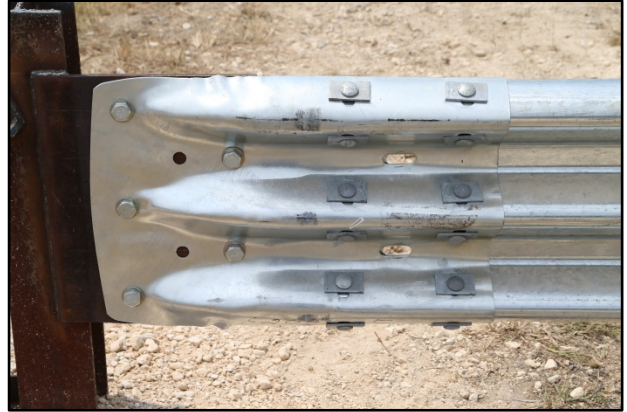
Figure 4.10. End Shoe before Test No. 490025-6 P4.
