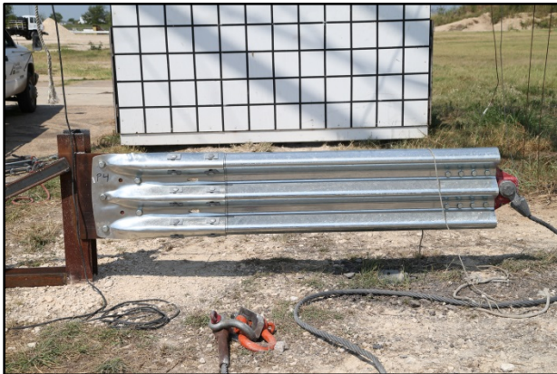
Figure 4.11. End Shoe after Test No. 490025-6 P4.
