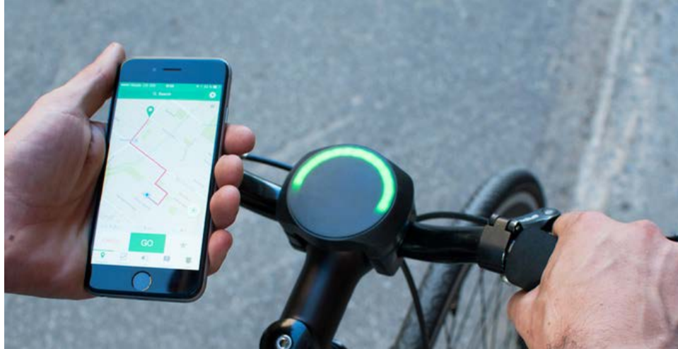
Figure 13. Possible Ways to Communicate Warning Messages to Bicyclists: SmartHalo Simplified Dashboard Paired with Smartphone.
