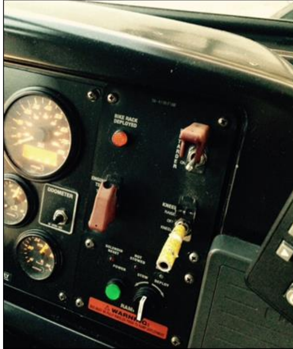
Figure 33. Bike Rack Deployed Indicator in a Gillig Bus.
