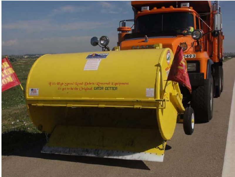
Figure 2. Gator Getter Mounted on a Colorado DOT Truck (Strong and Valdes-Vasques, 2014).
