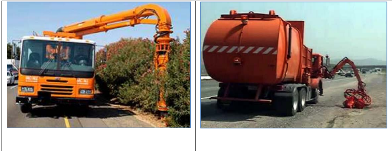
Figure 1. Automated Road Debris Vacuum (Left) and Liter Bag/Debris Vehicle (Right) (Strong and Valdes-Vasques, 2014).
