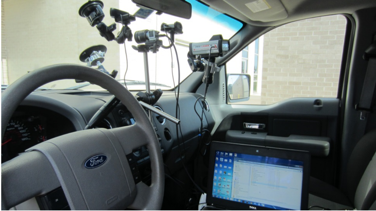
Figure 24. Setup for System Developed in Previous Study to Estimate Distance to a Leading Vehicle.
