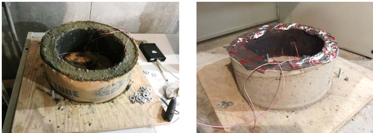
Figure 42. Ring Test: Concrete Ring at Age of 1 Days (Left) and at Age of 28 Days.
