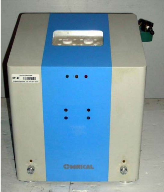
Figure 78. The Microcalorimeter Used in This Study.
