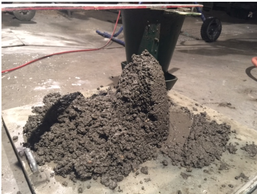
Figure 49. A Structural Collapse of the 0.45_520_100BRY/100BRY.
