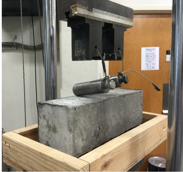
Figure 21. Flexural Strength Test.
