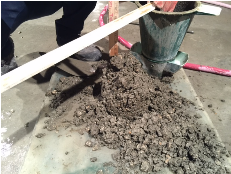
Figure 47. A Structural Collapse of the 0.40_520_100BRY/100BRY.
