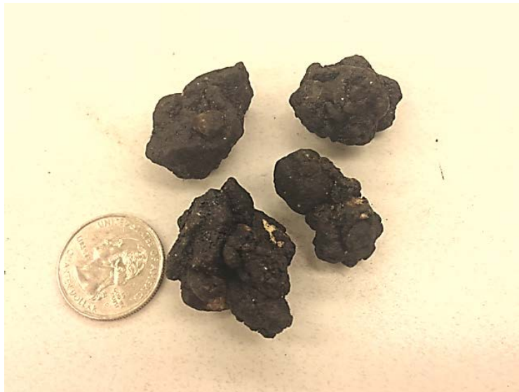
Figure 13. Agglomerated Particles in AMA_C.
