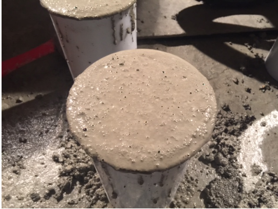
Figure 48 A Good Finished Surface of the 0.45_520_100BRY/100BRY.
