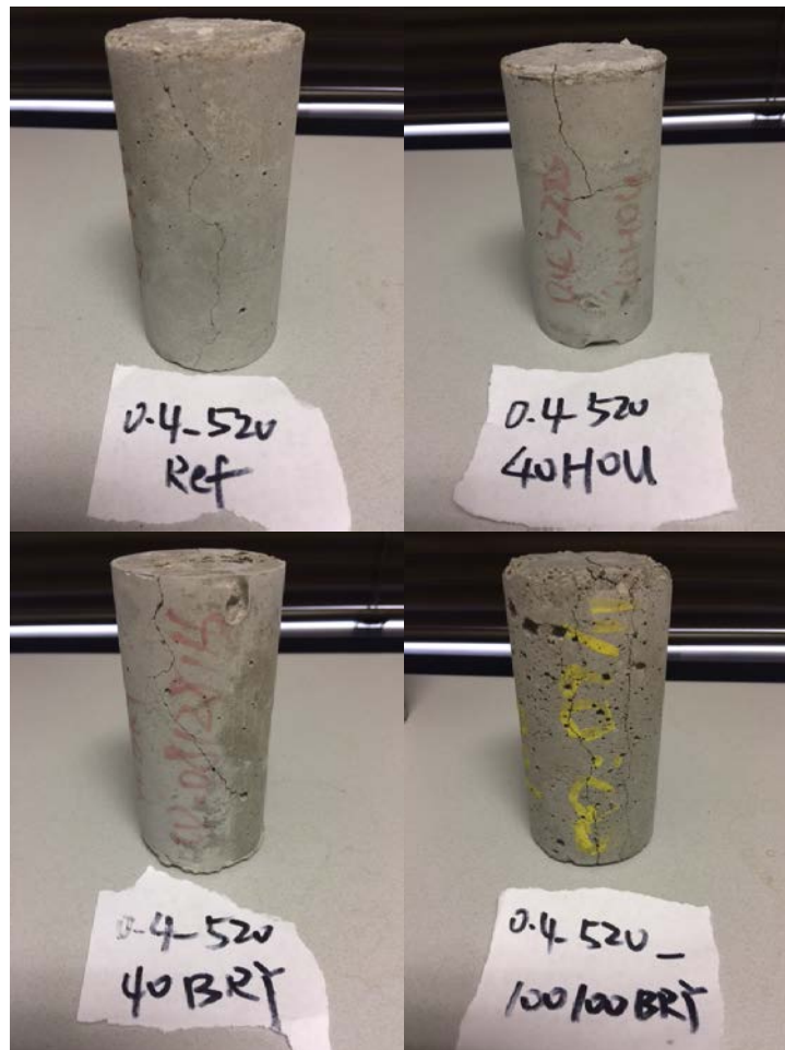
Figure 55. Cracked RAP-PCC Samples.
