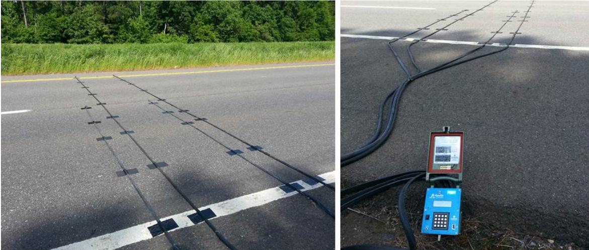
**Figure 27. Traffic Tubes and Counter/Classifier.**
