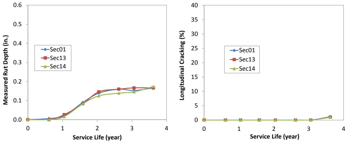
**Figure 17. Rutting and Longitudinal Cracking Performance of US 59 (Atlanta District).**
