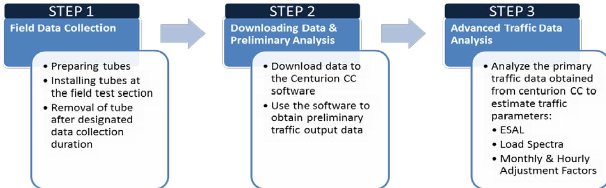
**Figure 26. The Steps Involved in Pneumatic Tube Traffic Data Collection and Analysis.**
