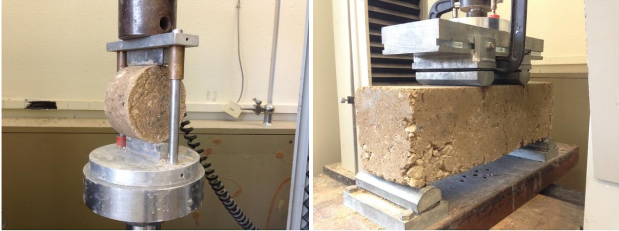
**Figure 15. Lab Mixed CTB Test: (a) IDT and (b) MoR.**
