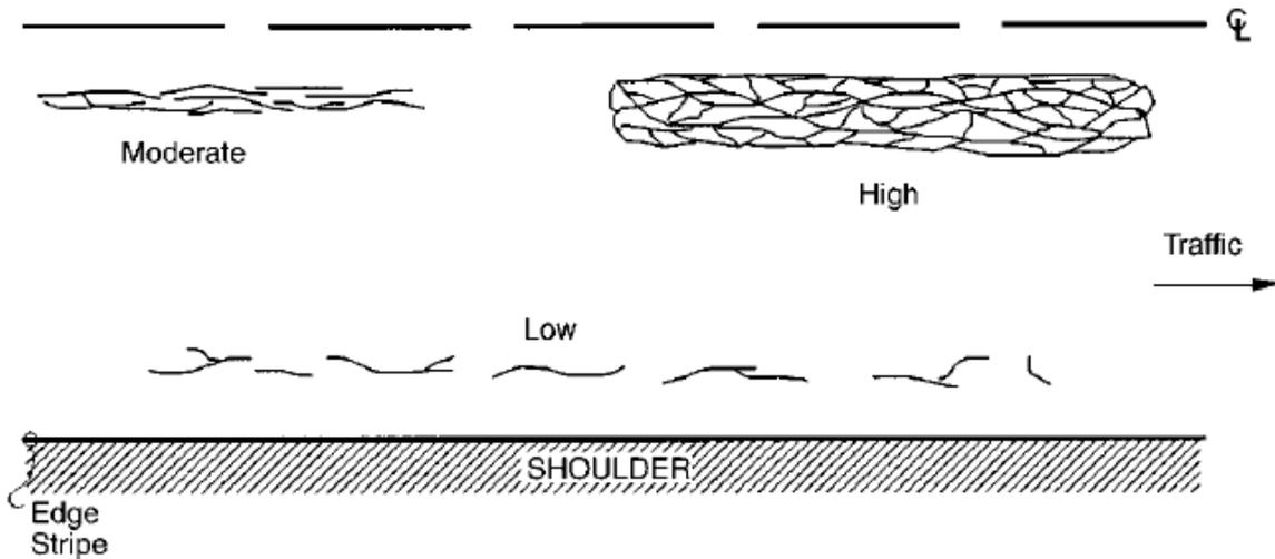
**Figure B-3. Severity of Alligator Cracking.**
