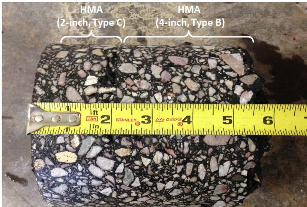
Figure 20. Cores from SH 304 after Construction (Austin District).
