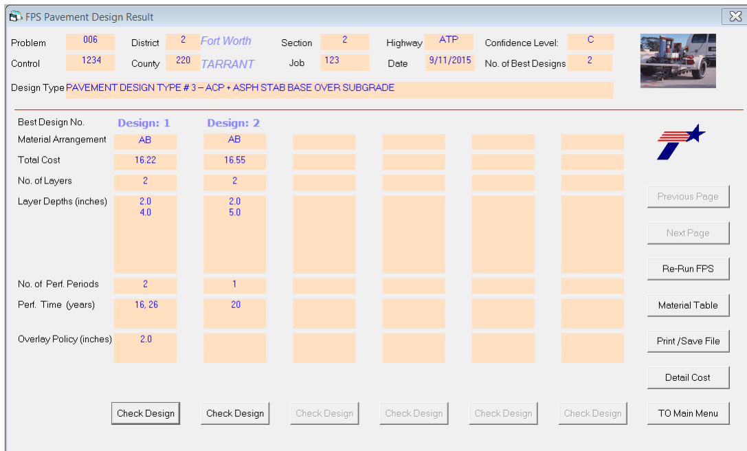
Figure 31. FPS Design Output: Pavement Design Result.
