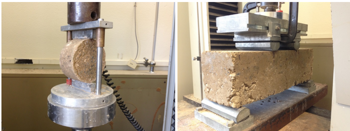
Figure 9. Lab-Mixed CTB Test: (a) IDT and (b) MoR.
