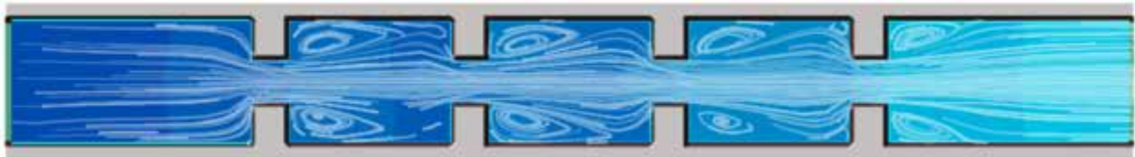
Figure 4.3: Representative Plan View from HEC-RAS 2D Showing Typical Flow Patterns from the Simulations (Flow Left to Right)
