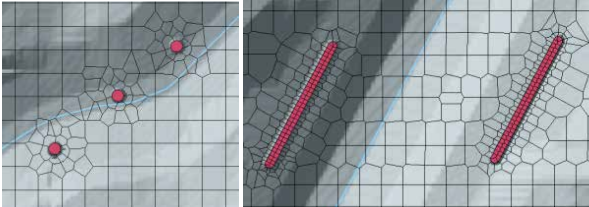
Figure 8.8: Mesh around Bridge Piers for Bridges 1176 and 1171
