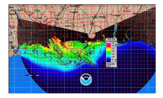
Figure 9. SLOSH Maximum Envelope of Water (MOM) Category Three Storm Projection
