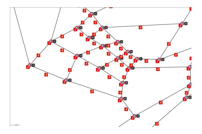
Figure 4. Urban portion of the network. Nodes labeled with degree ranking. Nodes labelled "1" most critical with 4 links connected.
