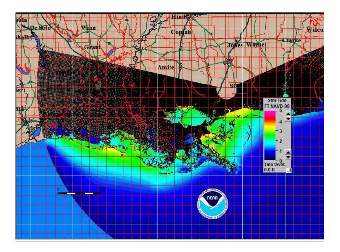
Figure 6. SLOSH Maximum Envelope of Water (MOM) tropical storm projection
