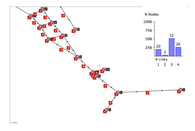
Figure 3. Coastal portion of network. Nodes labeled 4 have a single link attached, while nodes labeled 2 have 3 links attached. Inset is the histogram of the number of links per node for the entire network.
