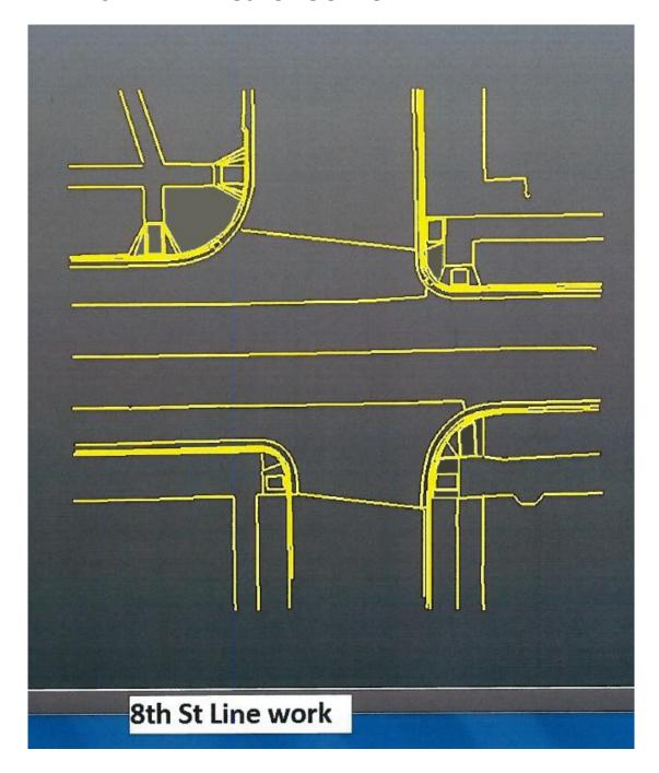
Figure 1: Contract No. 76H11, ADA ramps on US 50, linework for 8th Street generated from laser scanning data.
