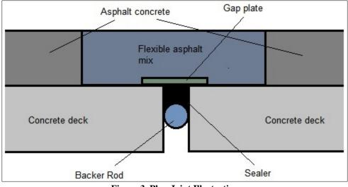
**Figure 3. Plug Joint Illustration**
