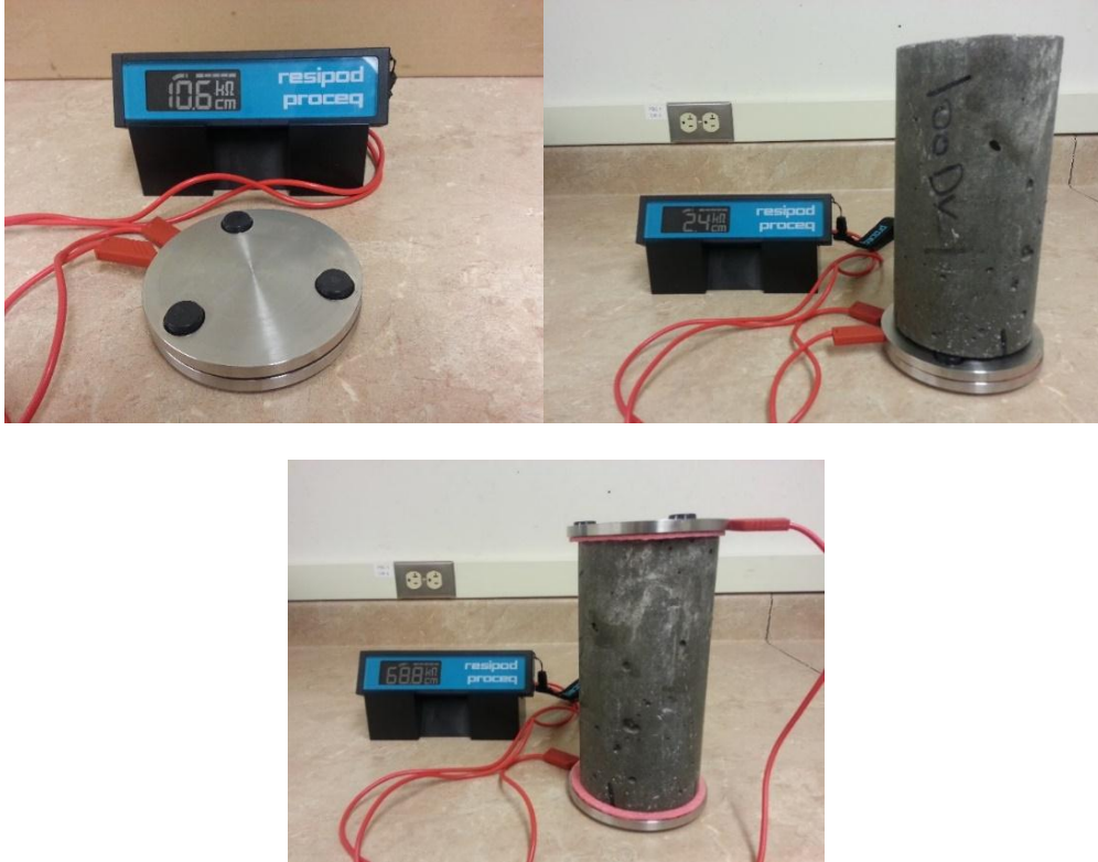
Figure 35- Measuring bulk electrical resistivity
