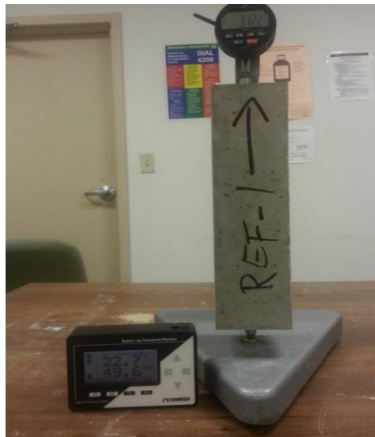
Figure 29- Length measurement for drying shrinkage
