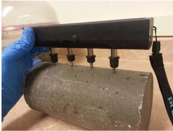
Figure 34- Surface resistivity measurement
