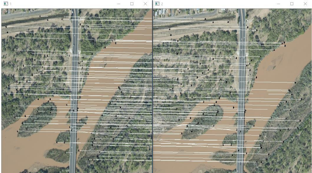
Figure 5.1: Result of feature-based image matching. Typically, the lines joining matches points are approximately parallel – this enables easy visualization of bad matches such as the one between moving cars near the bottom of the images.
