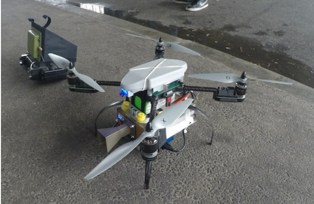
Fig. 57. Integrated CivilEye+Radar system
