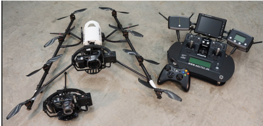
Fig. 5. Flight system Falcon UAV system with mounted digital camera Sony NEX 5 and additional camera Panasonic Lumix and mobile ground station (Hallermann and Morgenthal 2014)
