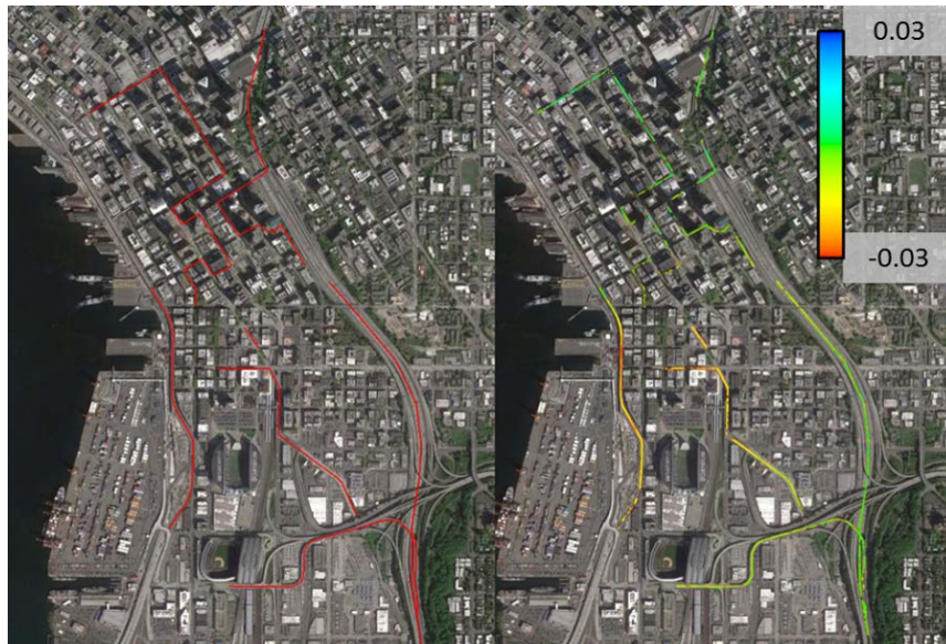
Figure 6-5 Example of defining arbitrary transects in a KML file and extracting the corresponding deformation map.
