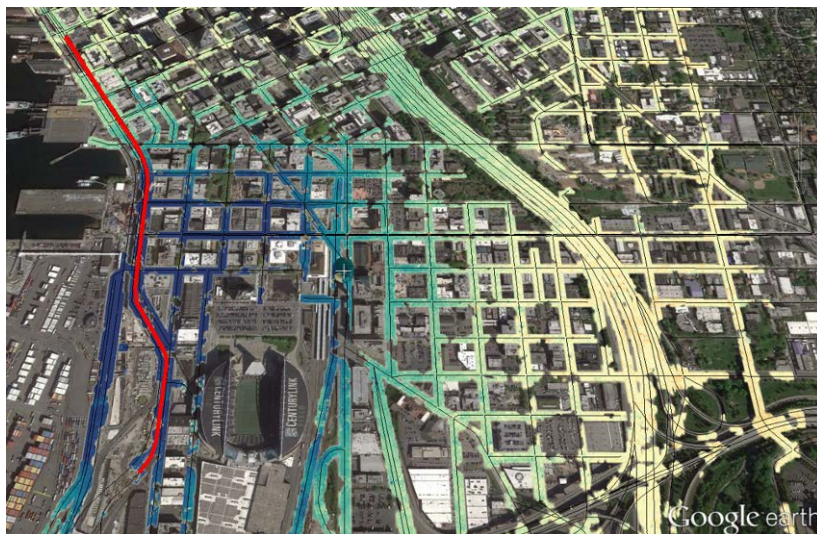
Figure 6-9 Example of extracting the deformation data on the Seattle road network, with overlaid KML lines which are selectable Google Earth features (red line).
