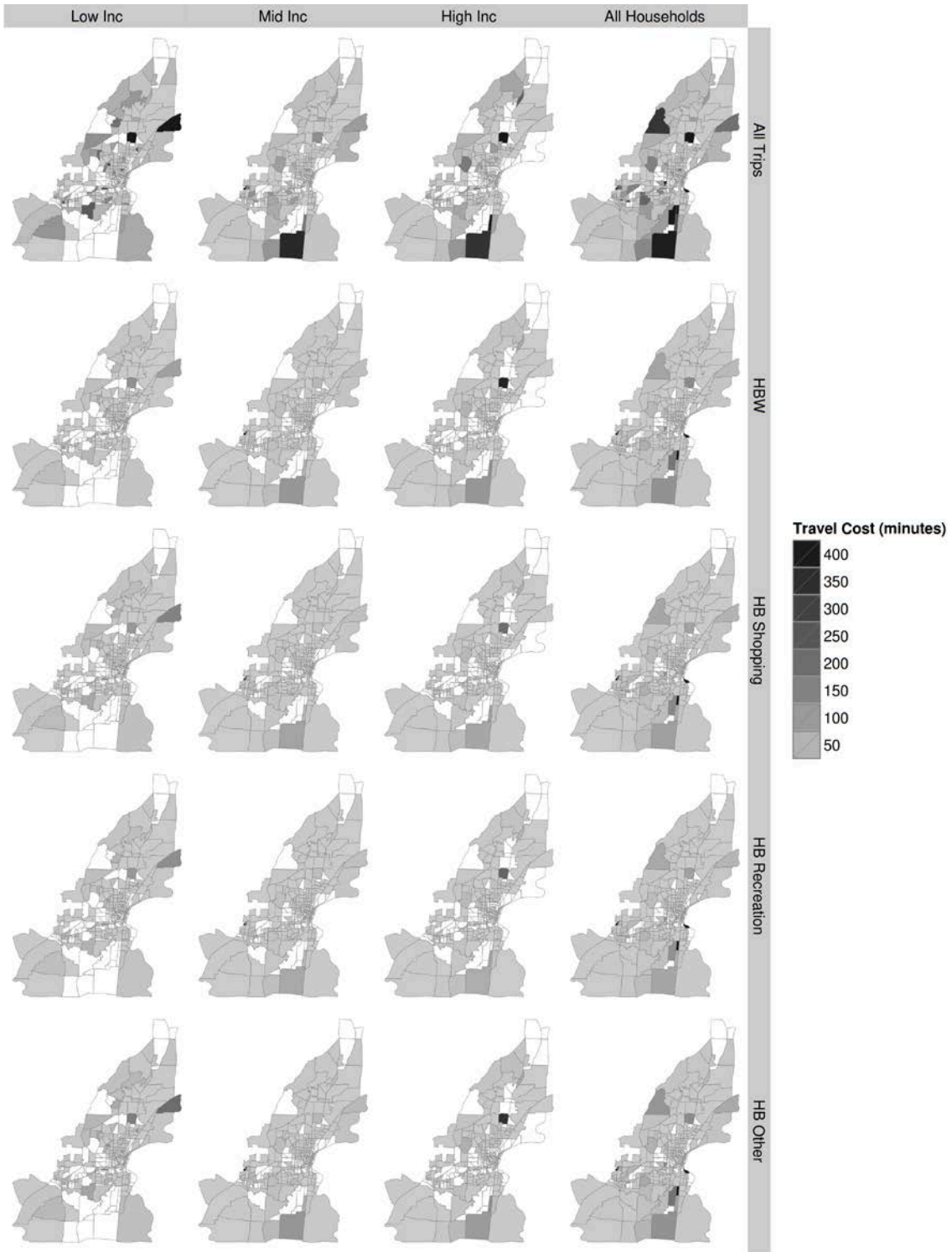
Figure 6.10: TAZ-level travel costs by income level and trip purpose for Corvallis Scenario A (halving auto travel time; leaving all other data unchanged from the 2010 CAMPO JEMnR model)
