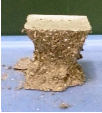
Figure 2.4-4–Representative failure mode of compression test cubes
