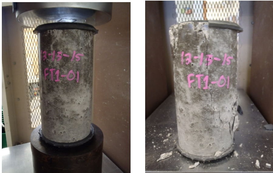
Figure 3.2-1–Concrete cylinders before and after compression test
