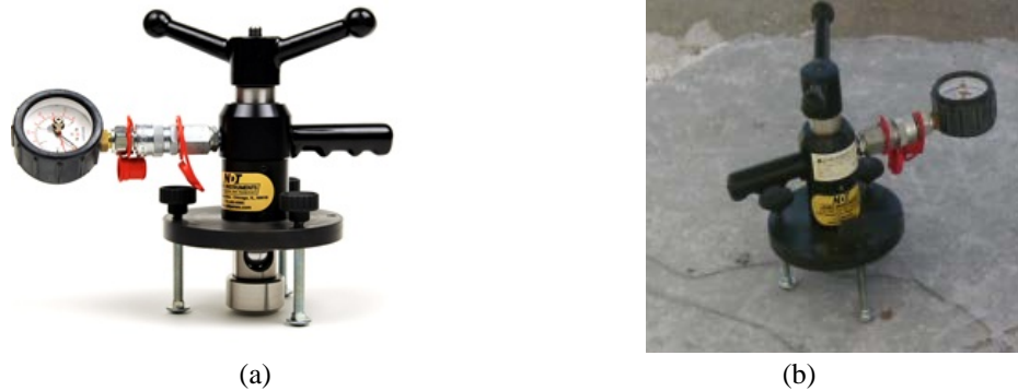
Figure 2.4-13 –Pull off test instrumentation: a) James Bond tester; b) test set up
