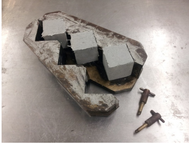
Figure 2.4-1–Cube de-molding for compressive strength of mortar tests
