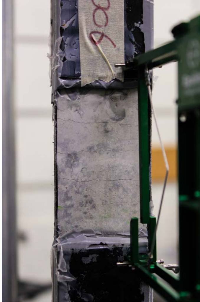
Figure 2.4-8 – Crack propagation in tensile coupons
