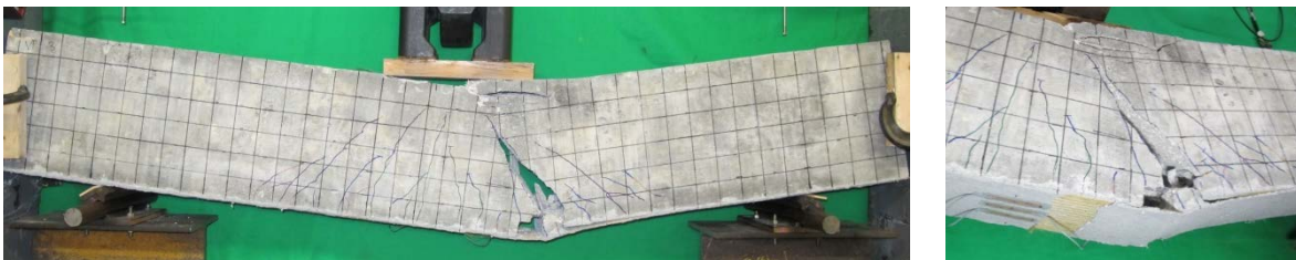
Figure 3.7-8– Typical fatigue failure mode for Phase II beams
