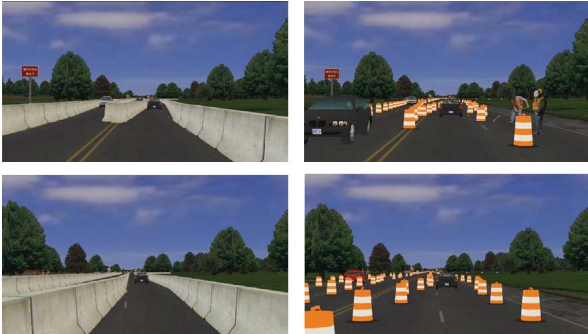
Figure 4-2: Left: High Level of Lane Configuration Factor for PCB; Right: High Level of Lane Configuration Factor for Work Drums
