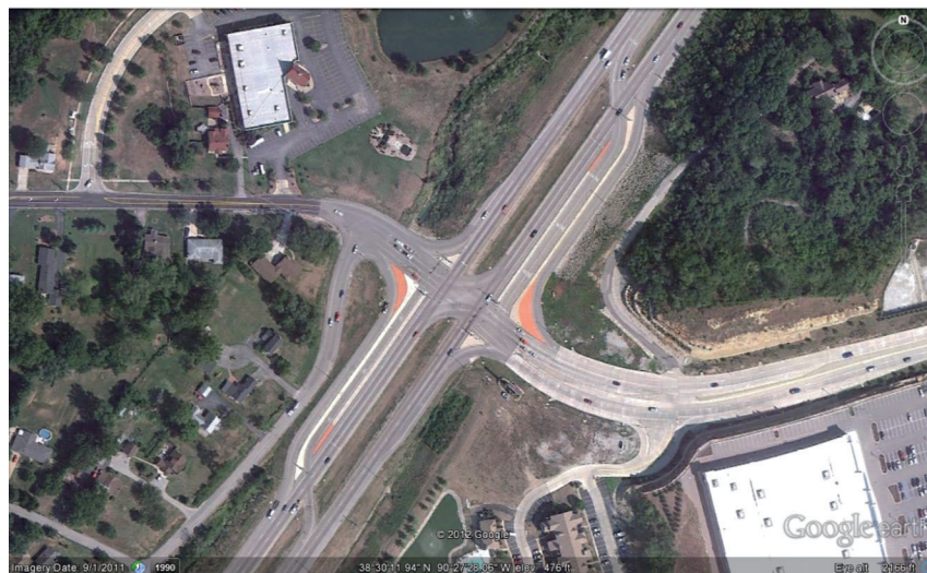
Figure 6.7 Partial DLT at Missouri Route 30 and Gravois Bluffs Blvd. in St. Louis, MO (27).
