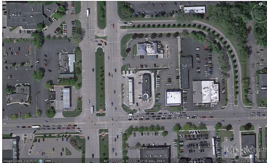
Figure 6.10 Partial QR at Telegraph Rd. & W. Maple Rd. in Broomfield Hills, MI (28).
