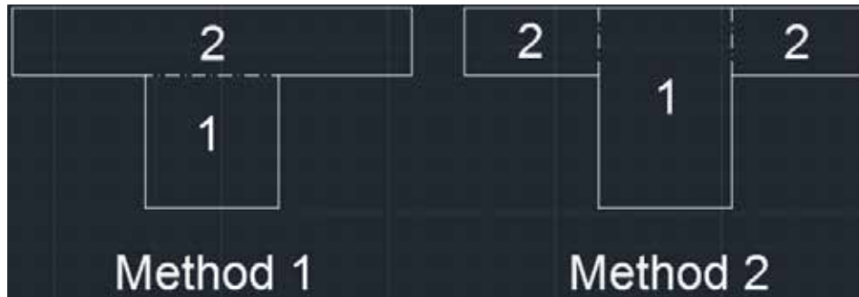
Figure 3.14: Methods to Calculate the Torsional Constant
