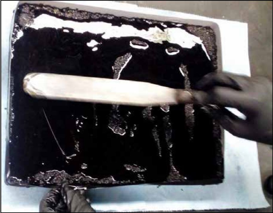
Figure 3.14: Epoxy Application Over the Slab
