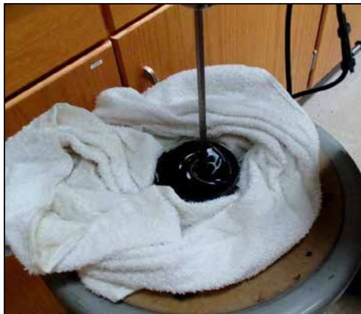
Figure 3.12: Mixing of Part A and B of the Epoxy
