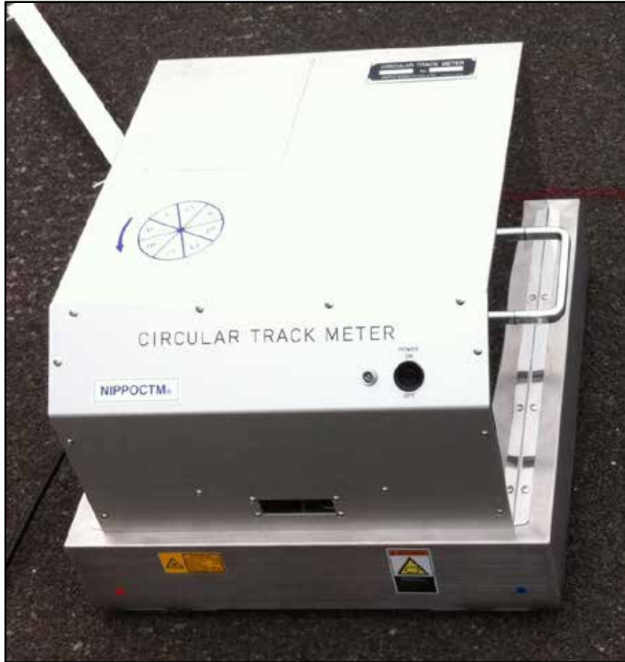
Figure 3.17: Circular Track Meter for Measuring Texture Depth
