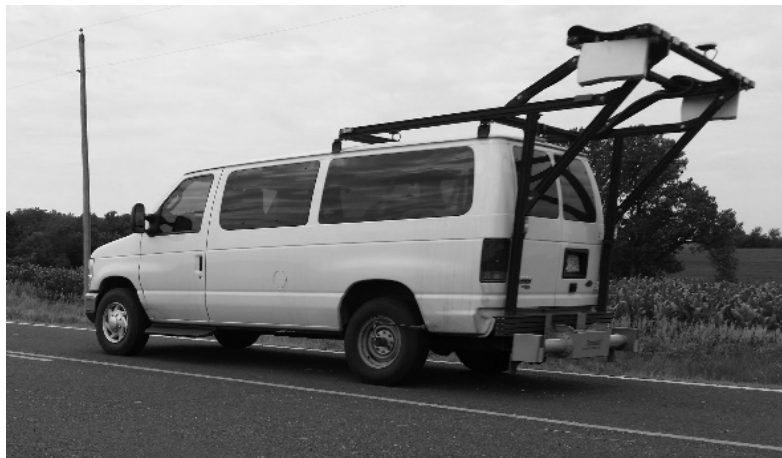
Figure 3.1: KDOT Laser Crack Measurement System Used in this Study
