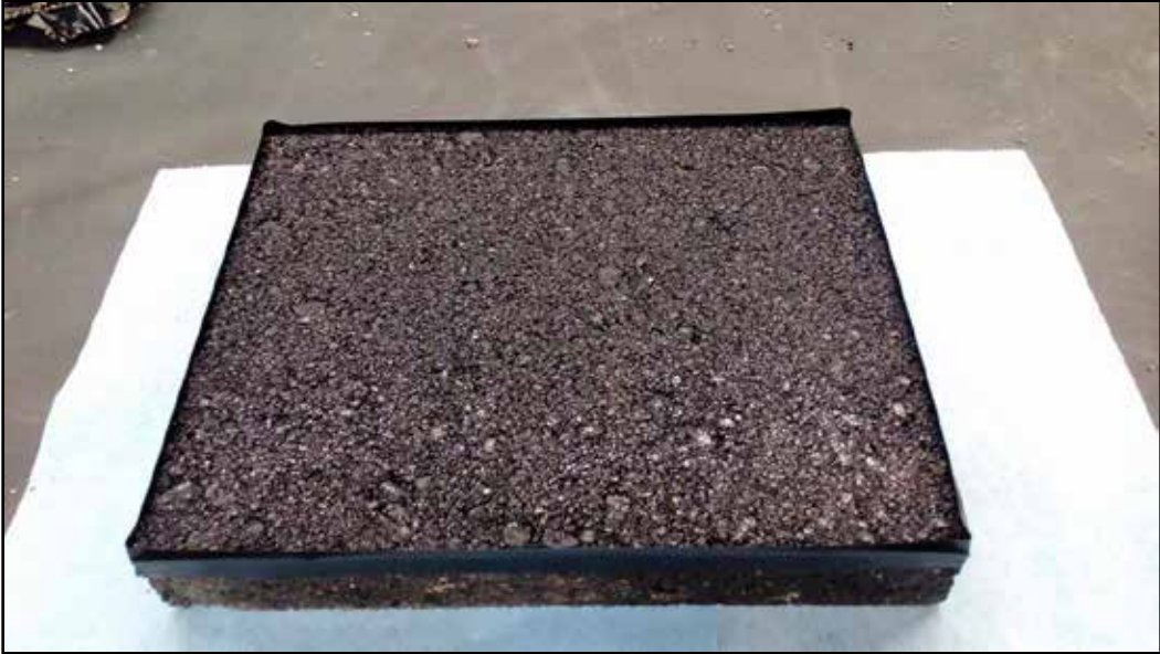
Figure 3.13: Duct Tape Applied on Sides of the Slab to Prevent Epoxy Loss
