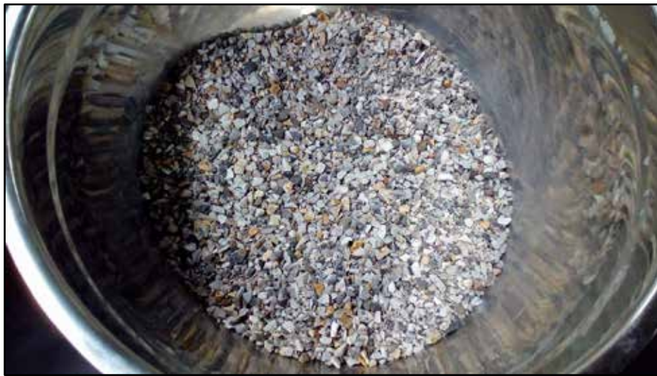
Figure 3.4: Picher, Oklahoma, Flint Aggregate Used in this Study
