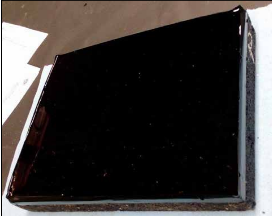
Figure 3.15: Slab Covered with Epoxy
