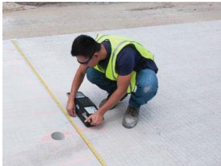
Figure 72: MIRA scanning for dowel locations near core.
