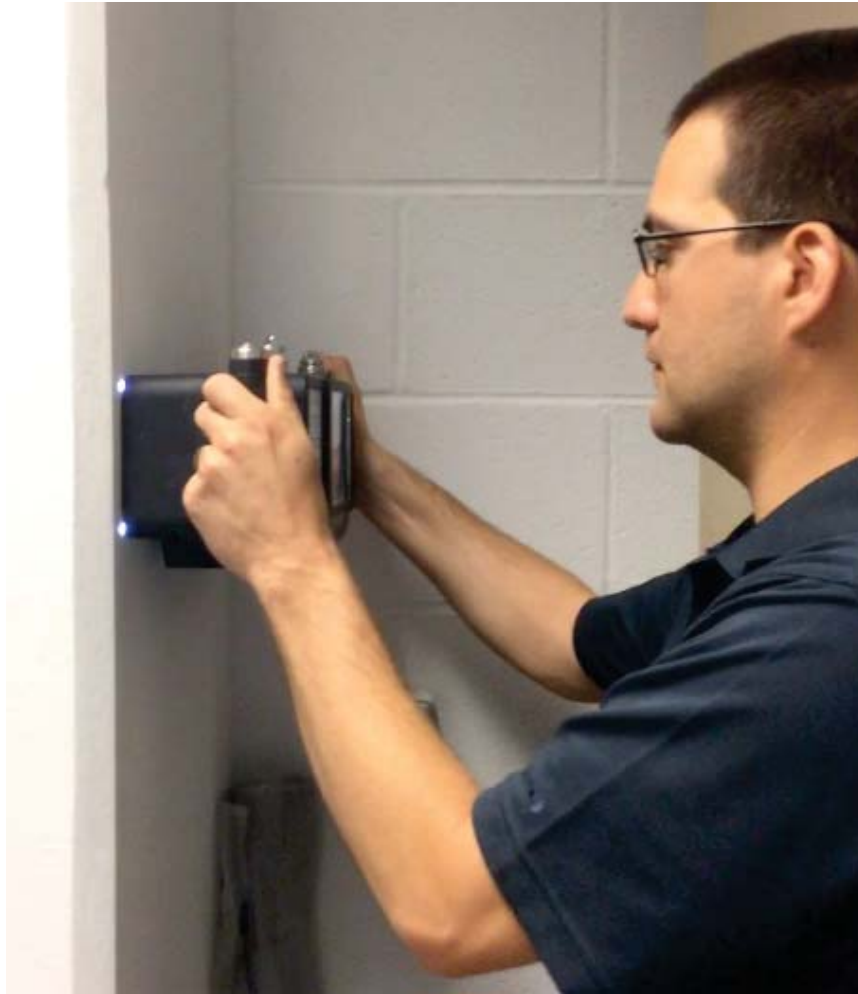
Figure 9: A photograph of a user pressing the MIRA firmly into place before taking a scan of a concrete segment.
