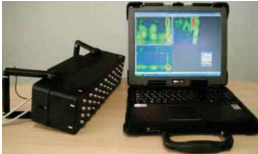
Figure 1: MIRA Ultrasonic Imaging Device and laptop with software (Germann Instruments 2010).
