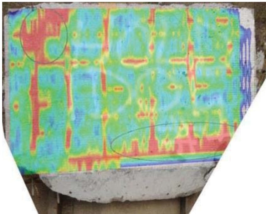
Figure 40: Map scan of delamination reflectors from 0 to 160 mm (0 to 6 in.) in Slab 1 transposed on top of a plan view photograph.
