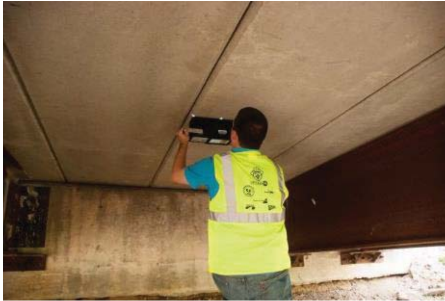
Figure 50: Photograph of scanning process on visually pristine double box girder. Orientation scanning perpendicular to traffic flow.
