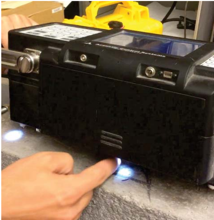
Figure 13: A photograph of the two lights on the underside of the device. These lights can be used to mark the concrete while in map mode. They are 170 mm (6.7 in.) apart.
