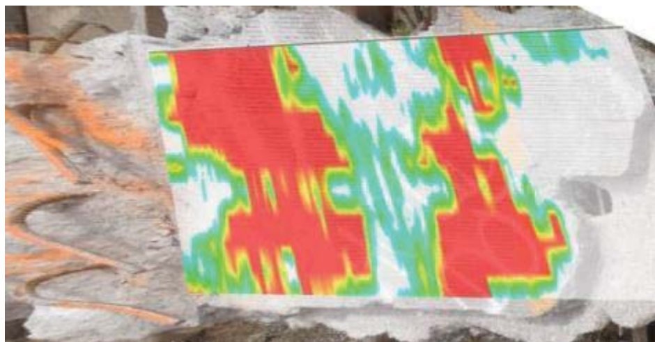
Figure 41: MIRA results plan view sliced from 0 to 160 mm (0 to 6 in.) for IDOT field bridge Slab 2.
