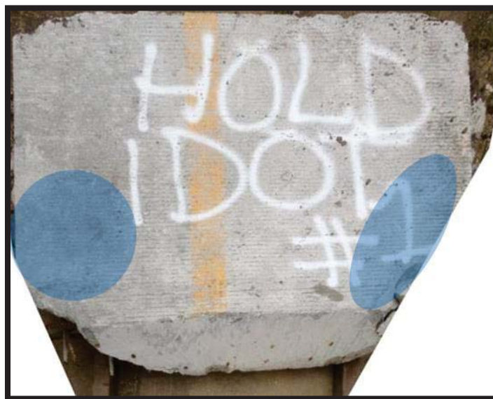
Figure 37: Sounding delamination results (highlighted in blue) for IDOT deck specimen Slab 1.
