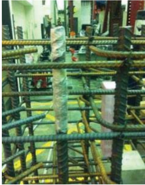
Figure 29: Simulated disbonding using a plastic-wrapped rebar during construction.
