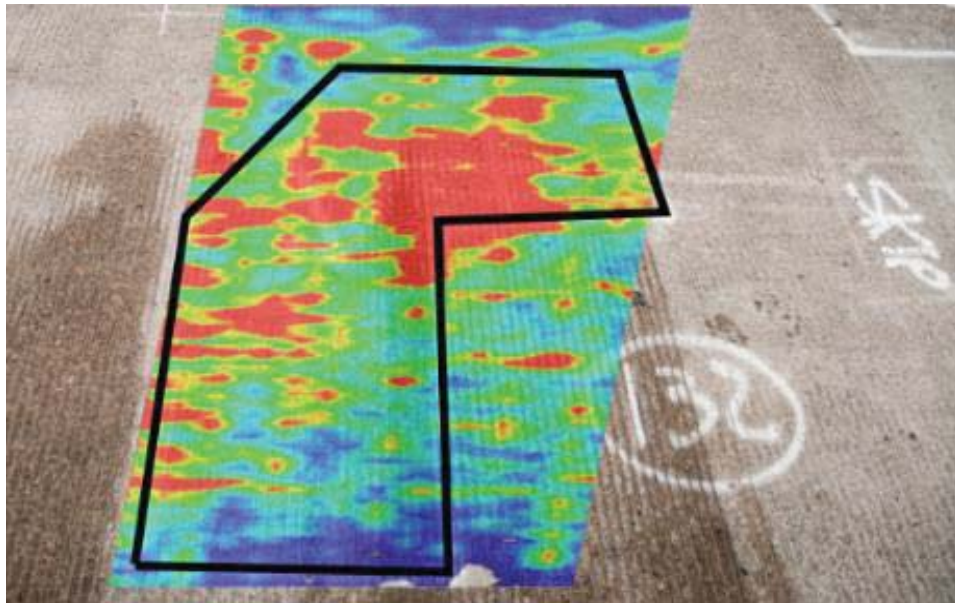
Figure 45: Near-surface reflectors in range 0 to 150 mm (0 to 5.9 in.) for the I-55 bridge deck delamination 132.
