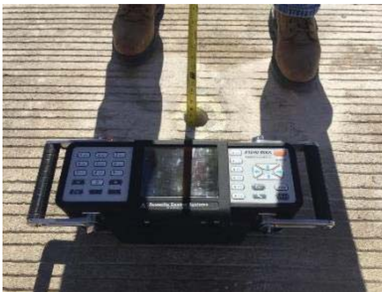
Figure 90: Measuring the thickness of a hole drilled through the slab.
