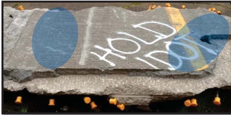
Figure 38: Sounding delamination results (highlighted in blue) for IDOT deck specimen Slab 2.
