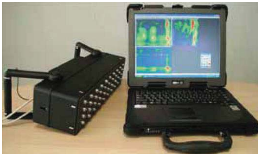
Figure 1: MIRA device and laptop. The device can connect wirelessly to the laptop to allow access in restricted areas (Germann Instruments 2010).
