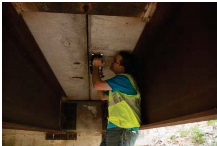
Figure 54: Photograph of visually corroded scan location and testing method.
