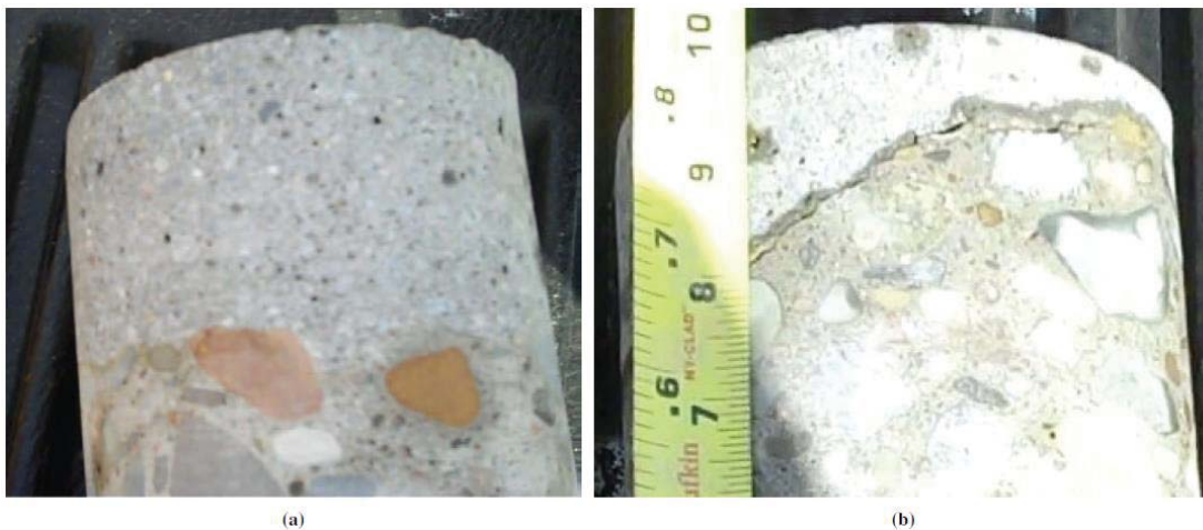
Figure 7: Cores taken from the locations tested in Hoegh et al. 2012. Figure 6 is core (a) and Figure 5 is core (b), imperial unit ruler shown (1 in. = 25.4 mm).
