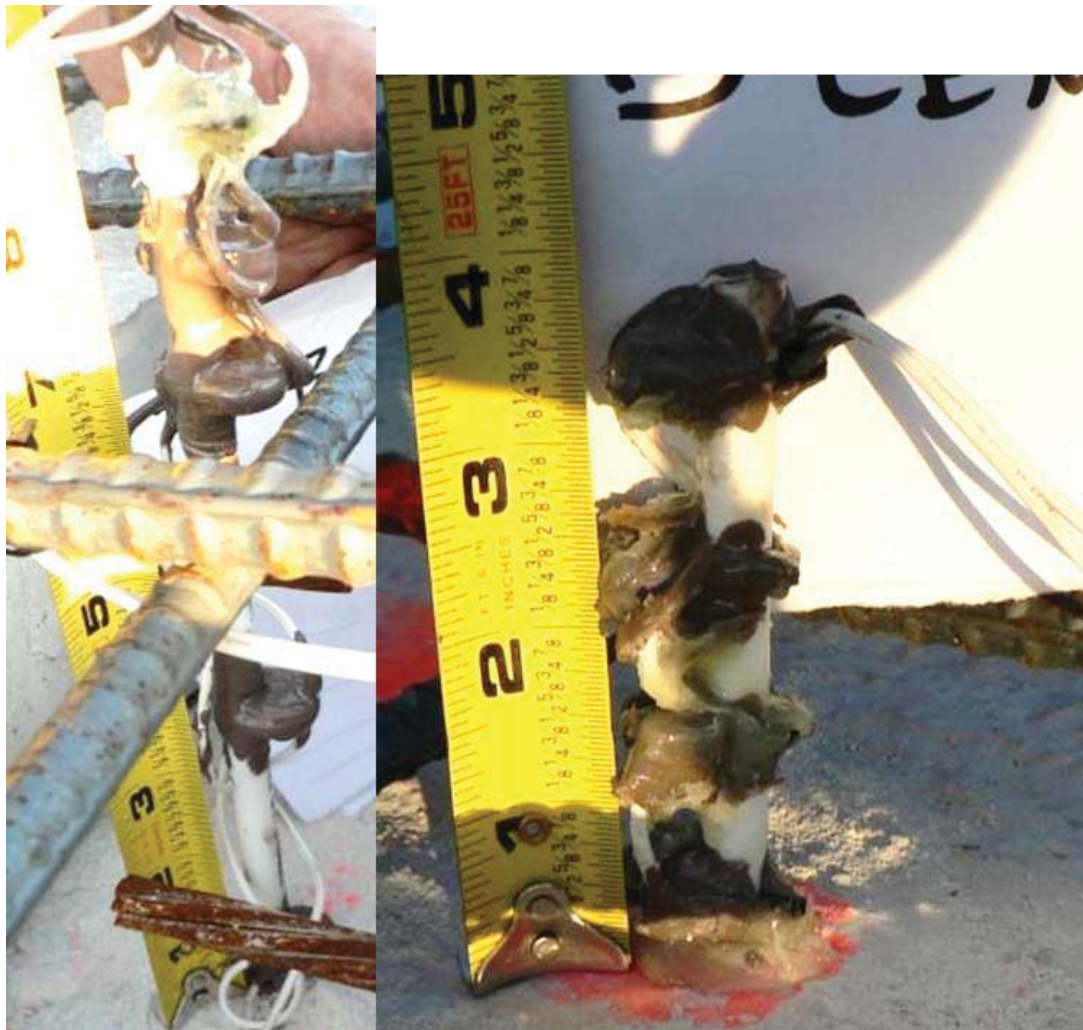
Figure 7.14: iButton strings on Georgetown bridge deck summer pour.
