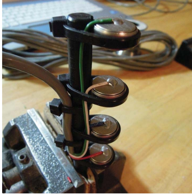
Figure 7.41: Sensor stick prior to epoxy coating.
