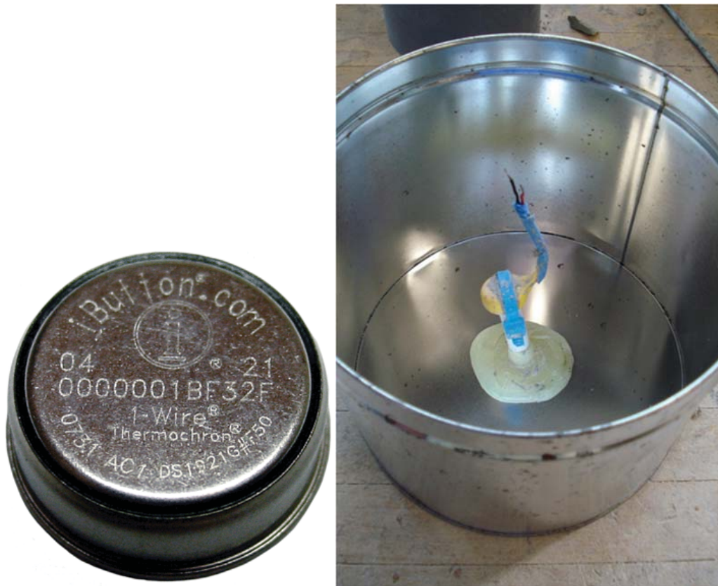
Figure 3.14: Temperature collection inside time-of-set can.
