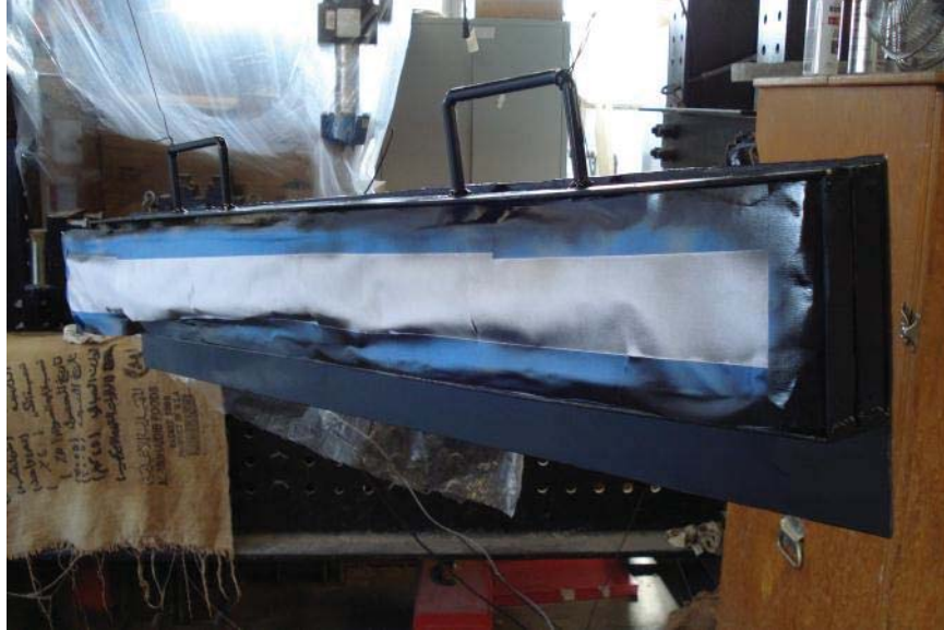
Figure C.8: Painting of steel formwork.
