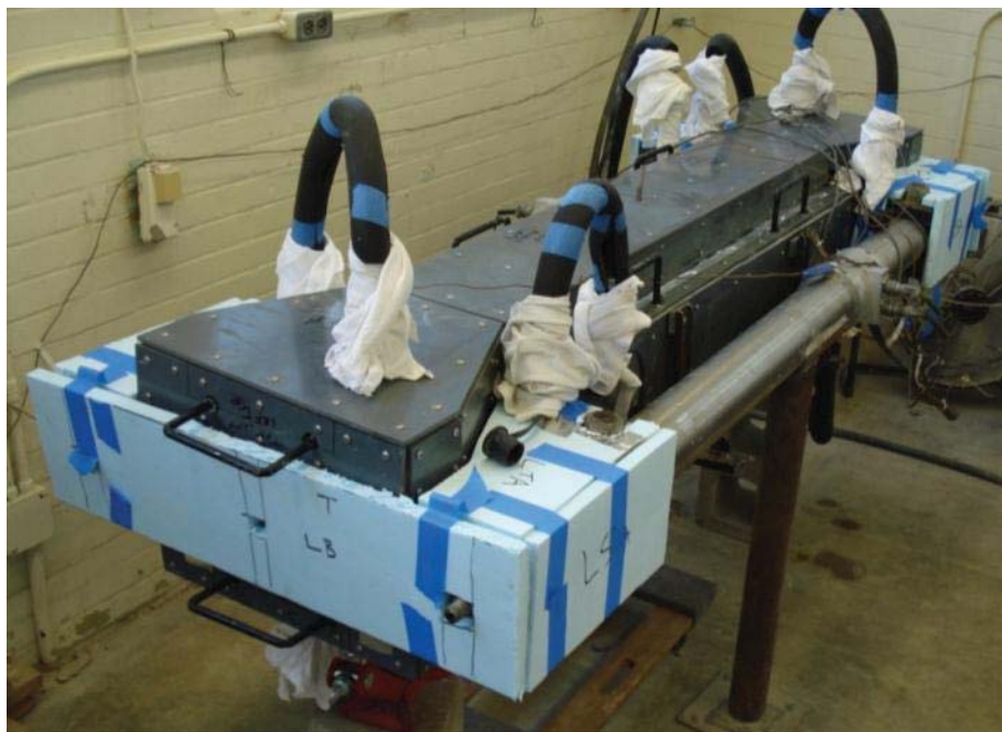
Figure 3.9: Rigid cracking frame with added insulation.
