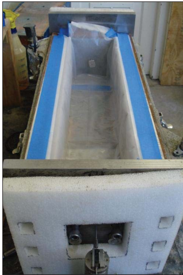
Figure 3.13: Free shrinkage frame after mix preparation.
