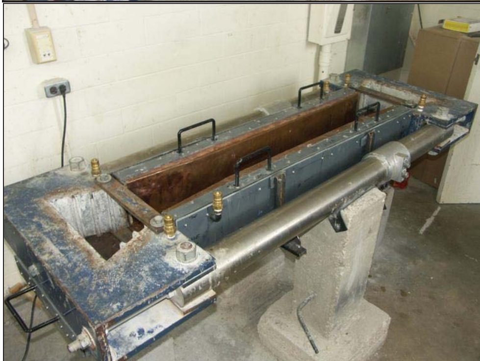
Figure 3.11: Rigid cracking frame with new formwork.
