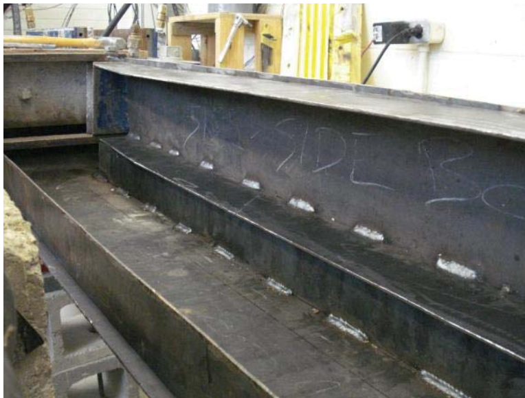
Figure C.5: Fitting of steel formwork.
