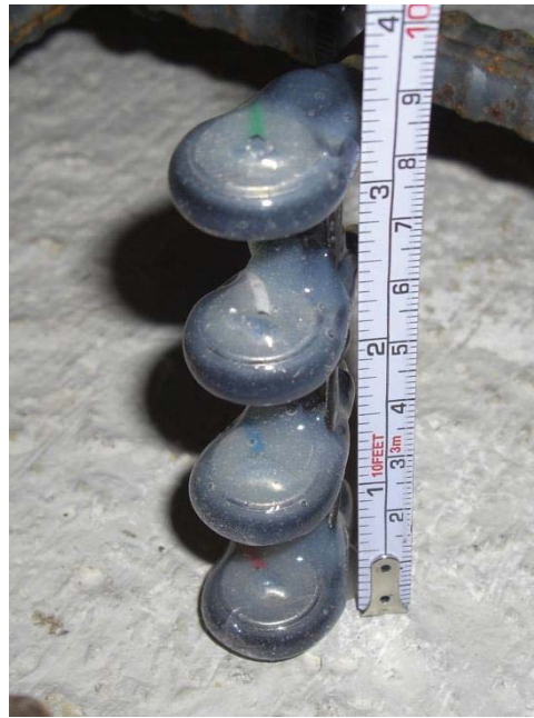
Figure 7.48: Installed temperature sensors.
