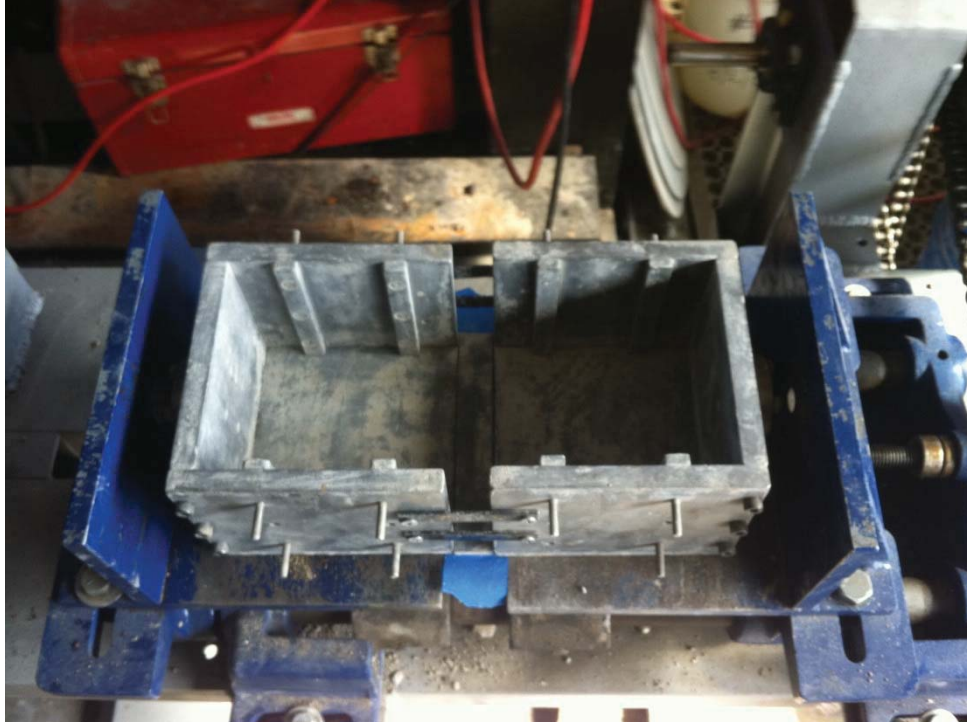
Figure 6.2: Direct tensile mold with PVC dowels.
