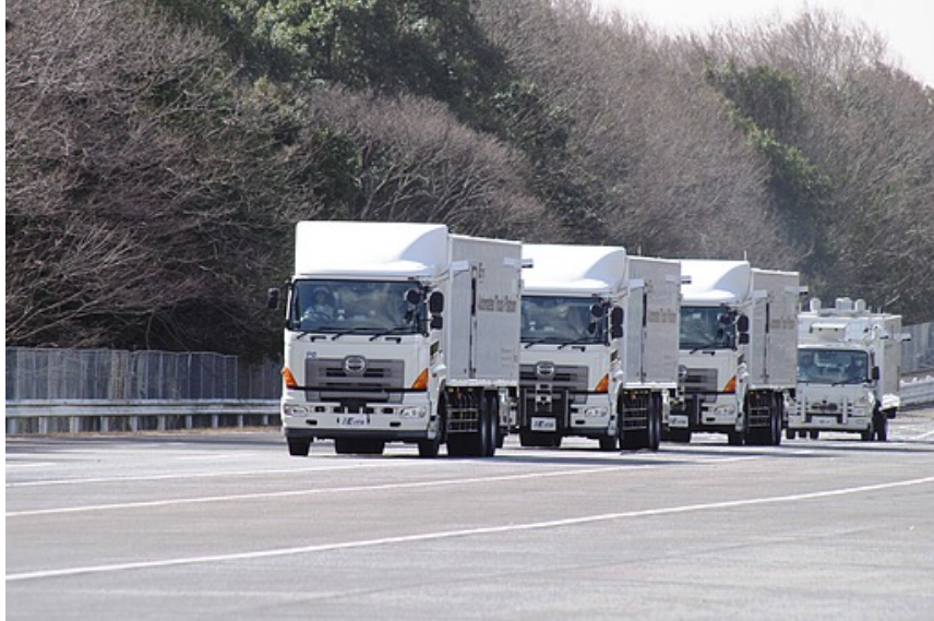
Figure 24. Four-Truck Platoon Demonstrated in Japan.
