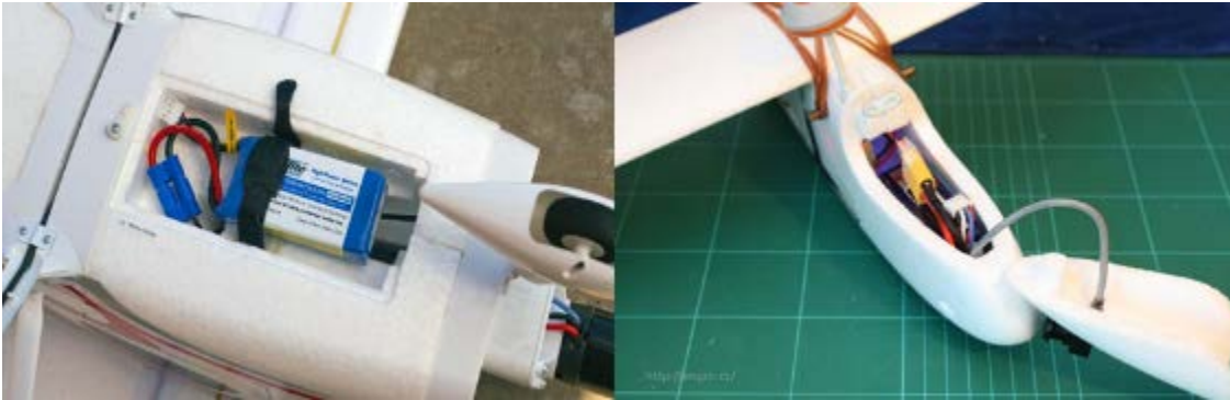
Figure D - 15 - LiPo battery Held Firmly inside FW UAS (left), LiPo Battery Mounted Loosely inside FW UAS (right)
