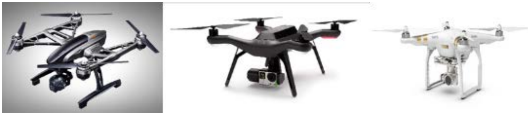
Figure D - 18 - Skid Landing Gear (left); Pointed Cantilever Landing Gear (center); Continuous Landing Gear (right)
