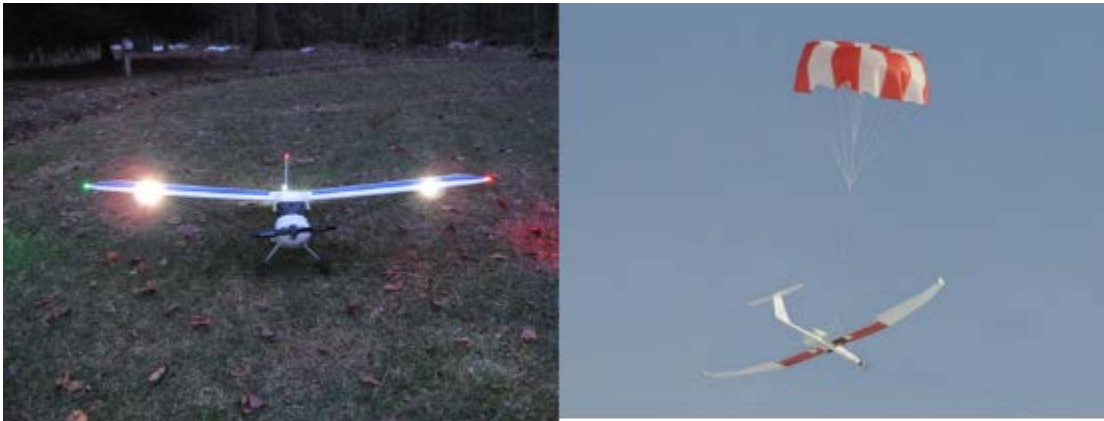
D-Figure D - 26 - Fixed Wing UAS with Landing and Position Lights (left) and Parachutes (right)
