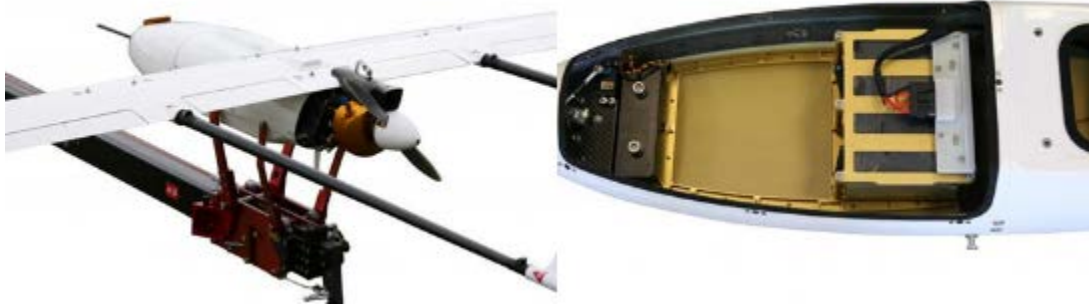
Figure D - 16 - Rear-Mounted Engine on a 50 lbs UAS (left); LiPo Batteries inside the Fuselage of a 33 lbs UAS (right)
