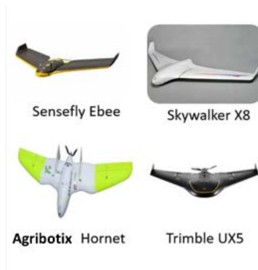
Figure D - 3 - Fixed Wing UAS with Flying Wing Configuration
