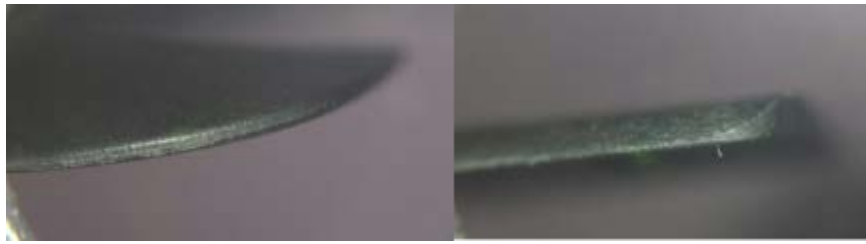
Figure D - 10 - Propeller with Sharp LE (left); Propeller with Sharp LE and Rounded Corners (right)
