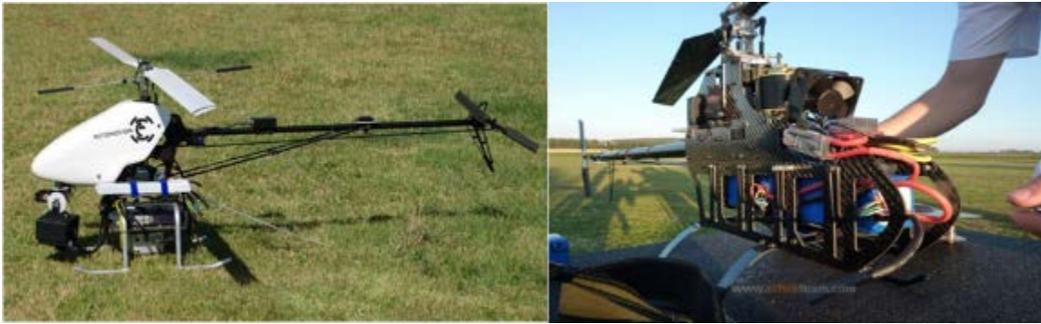
Figure D - 17 - Batteries on Side of Fuselage (left); Batteries inside the Fuselage Belly (right)
