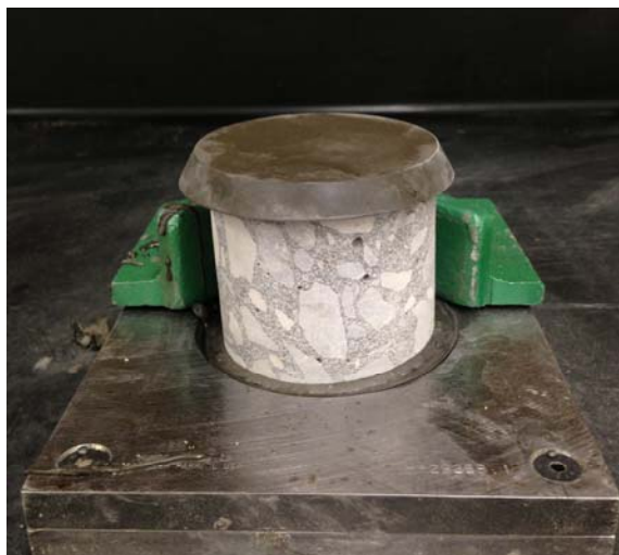
Figure 3-19: Modified capping stand for short cores
