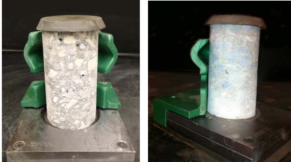
Figure 3-18: Example of sulfur capping
