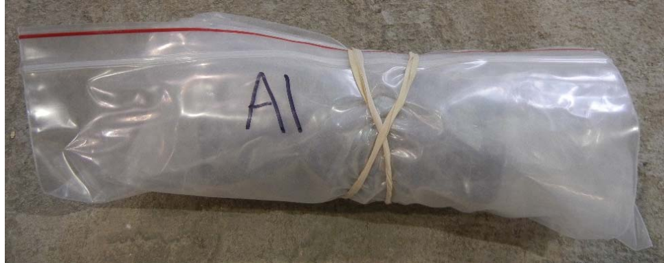
Figure 3-16: Core that has been bagged, rubber banded, and labeled
