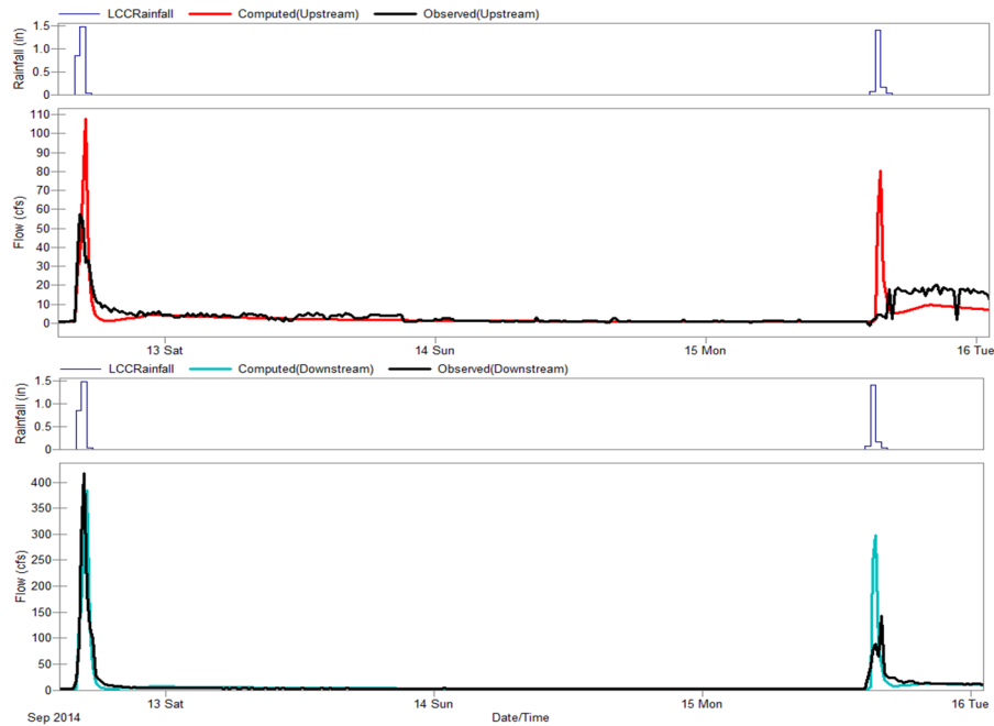
Figure 33: Flow hydrograph comparison for upstream (top) and downstream (bottom) simulated and respective measurements (9/12/2014).
