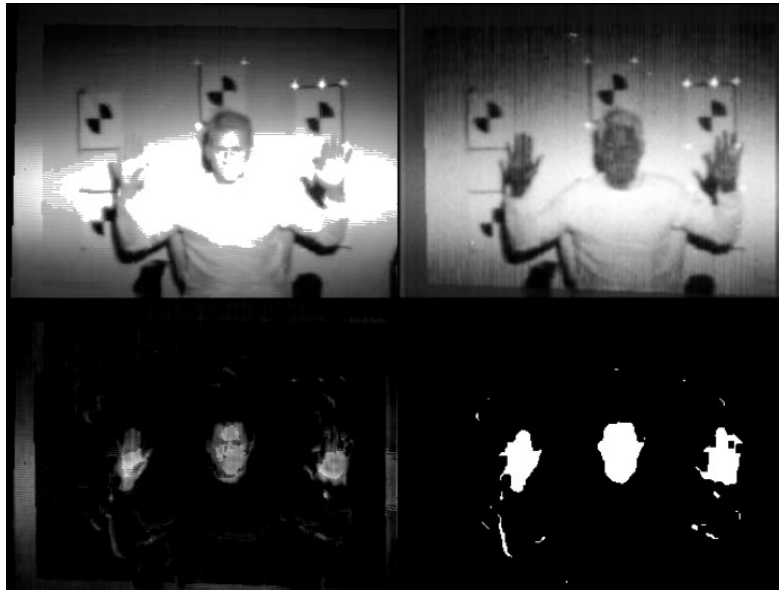
Figure 3.3. Human subject segmentation process. UPPER LEFT: Lower band < 1400 nm Image, I(u, v)_{Lower} ; UPPER RIGHT: Upper band > 1400nm Image, I(u, v)_{Upper} , LOWER LEFT: Difference Image, I(u, v)_D , LOWER RIGHT: segmentation binary image.
