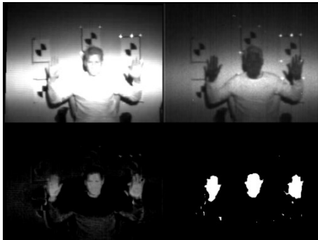
Figure 4.7. TBI human skin detection without window glass obstruction.
