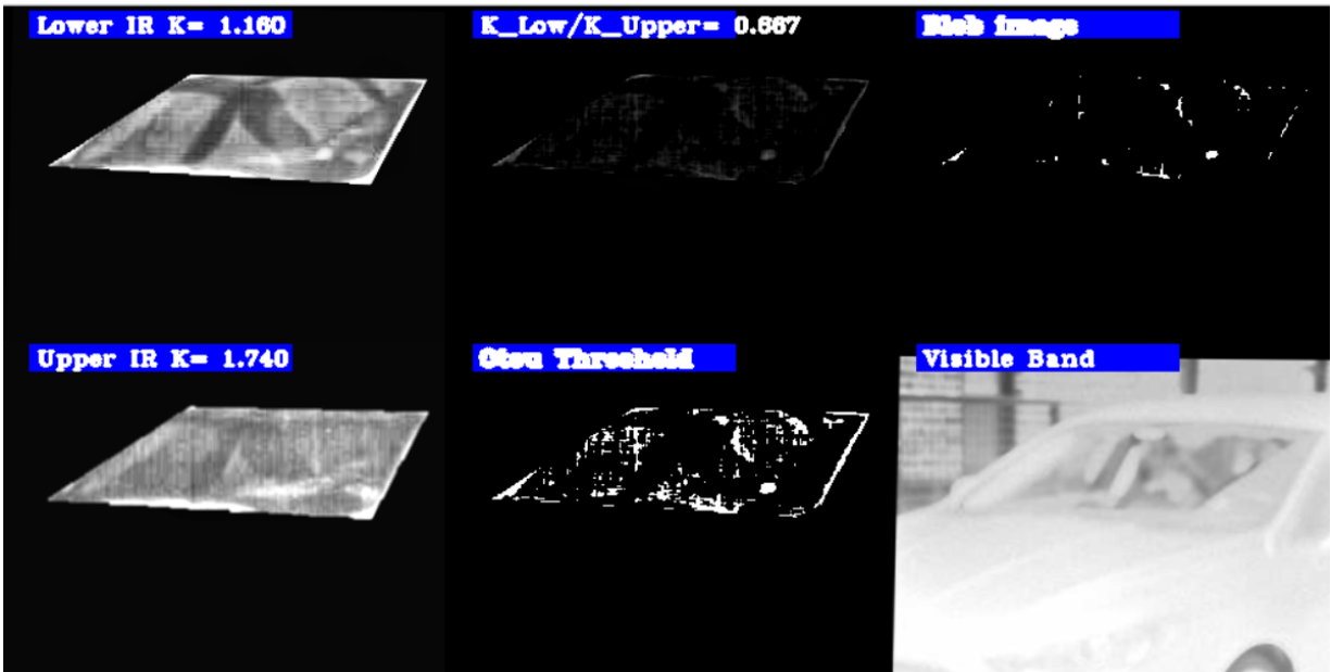
Figure 5.13. Ford 2016 Fusion, 15x6 sunny condition. Images clockwise from upper left: Lower band IR, Blob threshold, Upper band IR, binary threshold.
