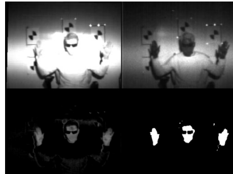
Figure 4.7. TBI human skin detection without window glass obstruction.
