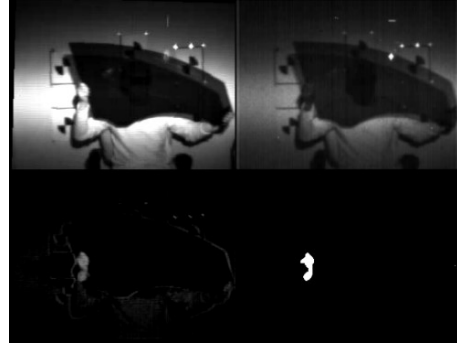
Figure 4.5. TBI human skin detection through Volvo S60 front passenger window.
