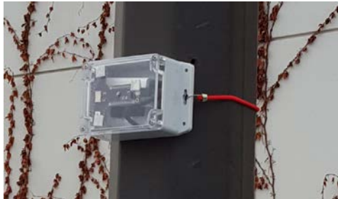
Bluetooth LE Module Attached to a Lamp Post (8-ft above ground)
