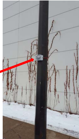
Figure 3-2 Placement of a Bluetooth Low-Energy Module on a Lamp Post
