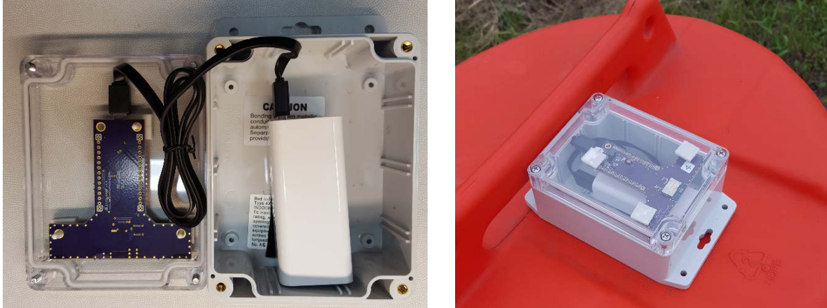
Figure 2-4 A BLE long-range module with battery packaged in a NEMA enclosure
