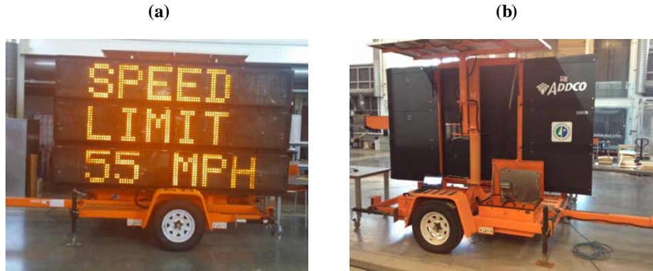
Figure 3.13 (a) Front and (b) Back views of the Variable Message Sign used in the development of the proposed system.
