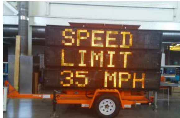
(b) Alternating Messages when worker is present in the field.
