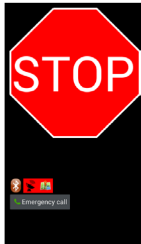
Figure 2.5. Stop sign violation visual warning
