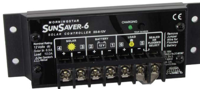
Figure 10: Morningstar SunSaver-6 solar charge controller.
