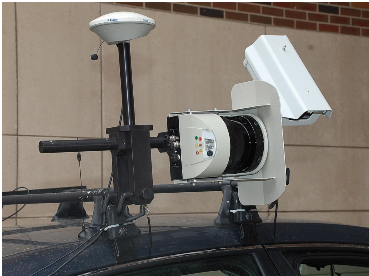
Figure 2.6: Vehicle mounts and sensor pod on Chevrolet Impala
