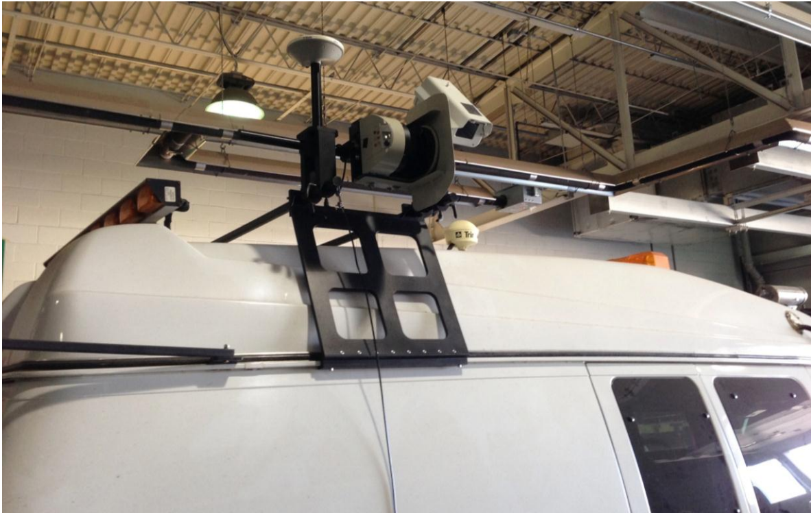
Figure 2.7: Vehicle mounts and sensor pod on Metro District's video logging van
