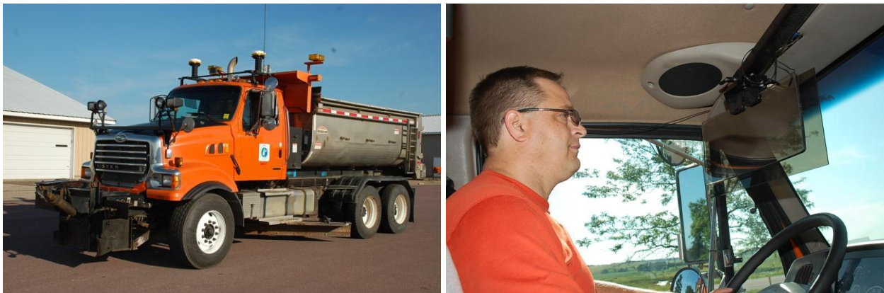
Figure 1.1: Instrumented snowplow and driver looking through HUD
